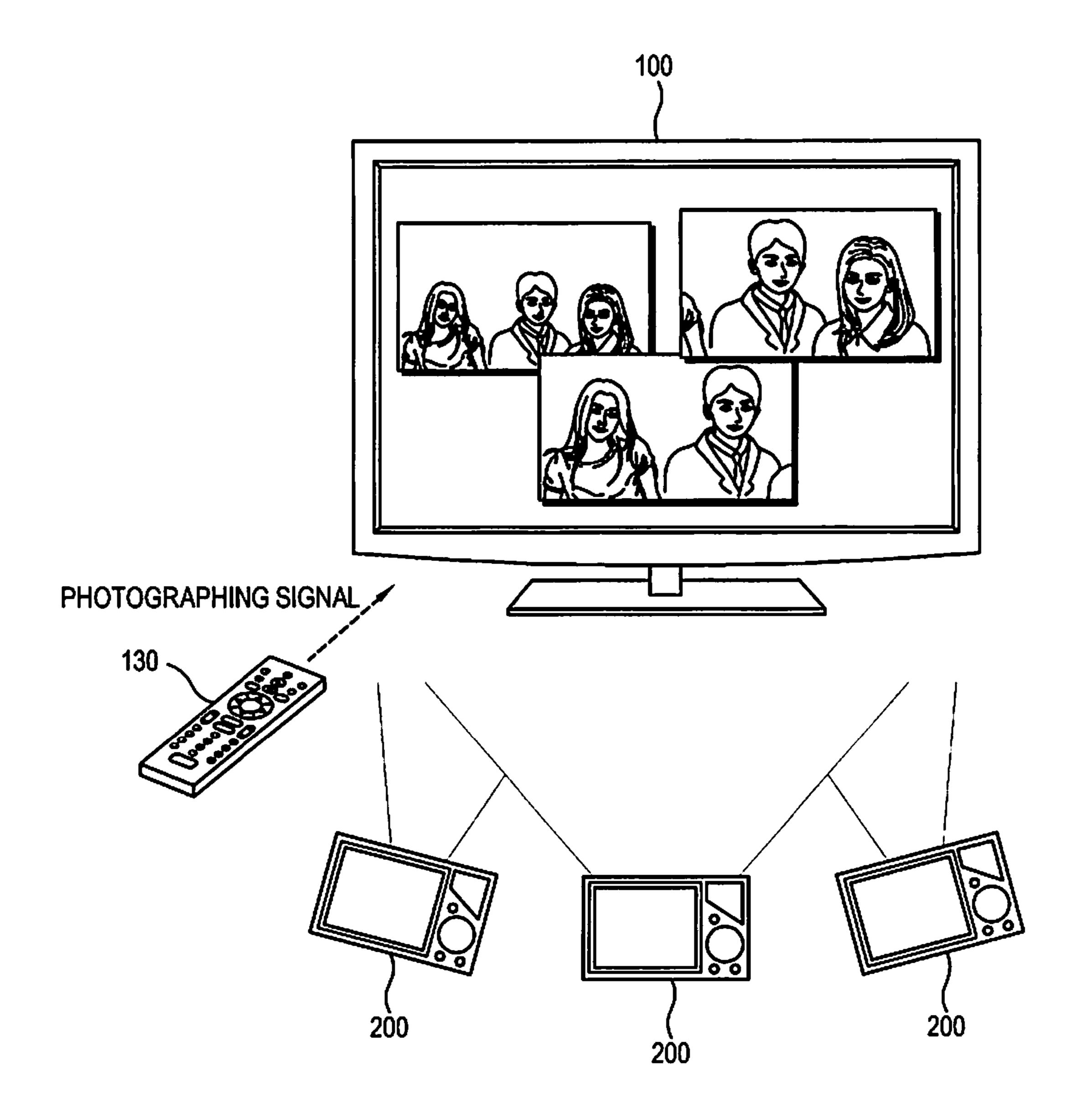
SECOND PHOTOGRAPHING UNIT COMMUNICATION UNIT **USER INPUT RECEIVER** FIRST COMMUNICATION UNIT FIRST CONTROLLER REMOTE ONTROLLER
