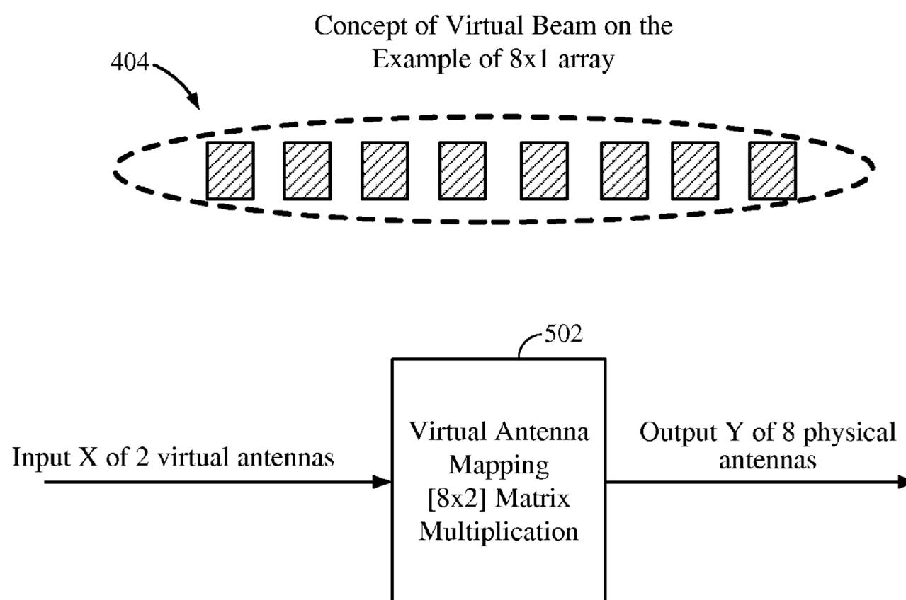
The virtual antenna mapping matrix can be updated with time or frequency to allow different virtual antenna mapping, e.g. different beam directions
