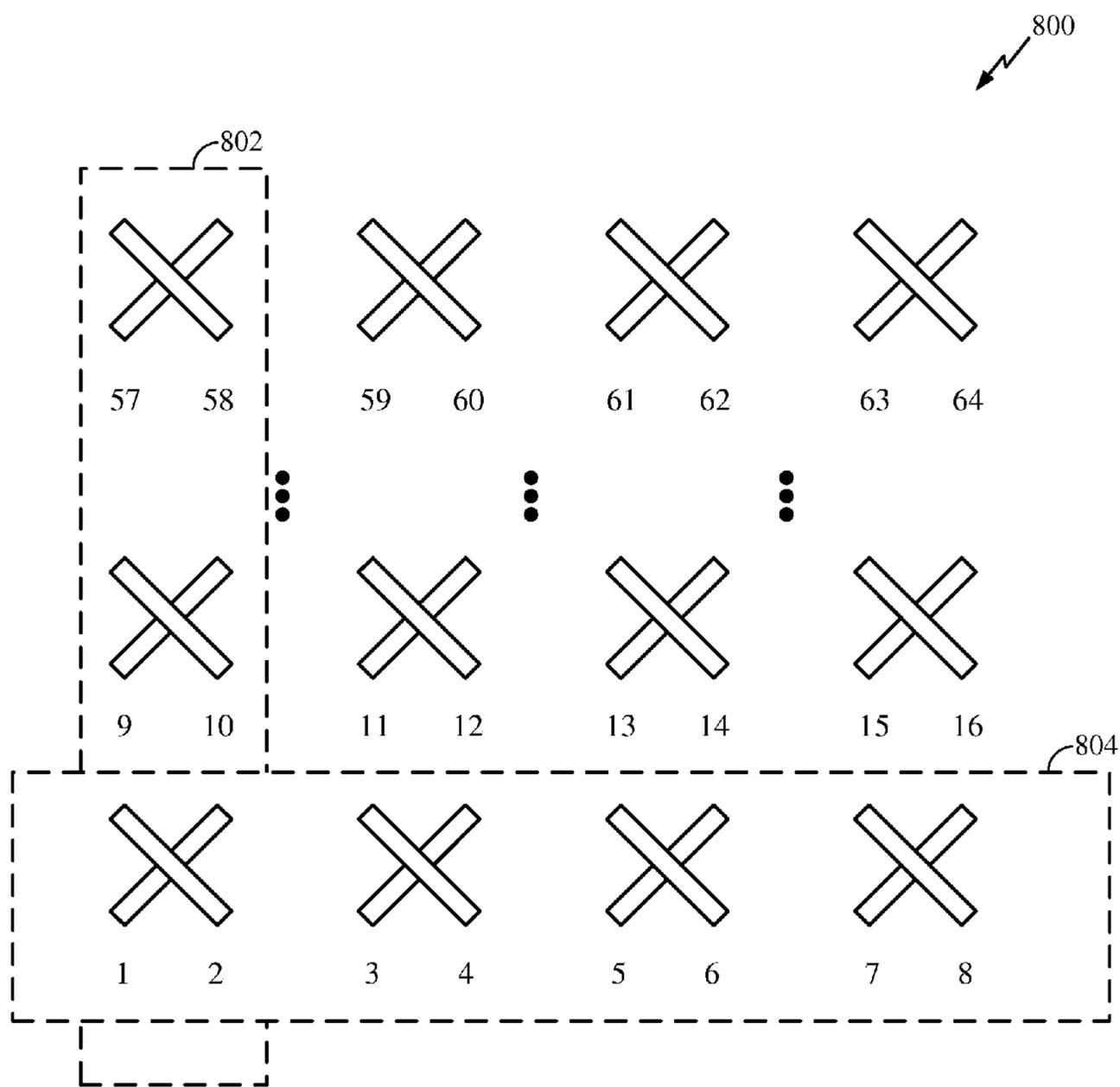
Ports 1, 2, 3, 4, ... 7 and 8 for azimuth PMI derivation
