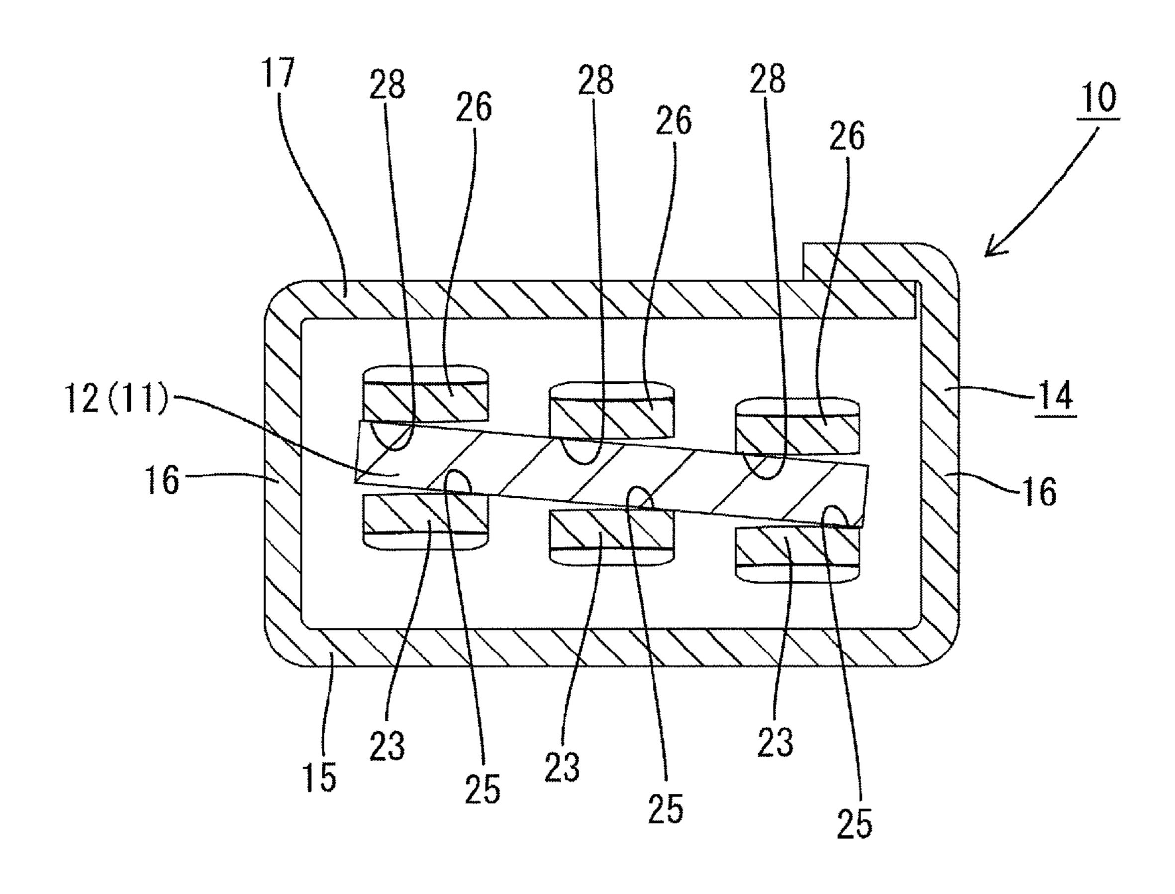
FEMALE TERMINAL HAVING OPPOSED FIRST AND SECOND PLURALITIES OF RESILIENT PIECES, WITH EACH RESILIENT PIECE HAVING A FREE END AND A CONTACT PORTION NEAR THE FREE END
