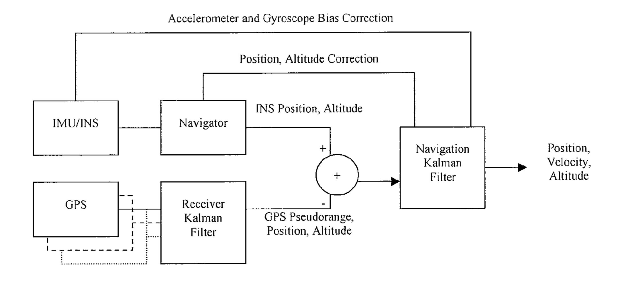
A tightly coupled GPS-IMU/INS system
