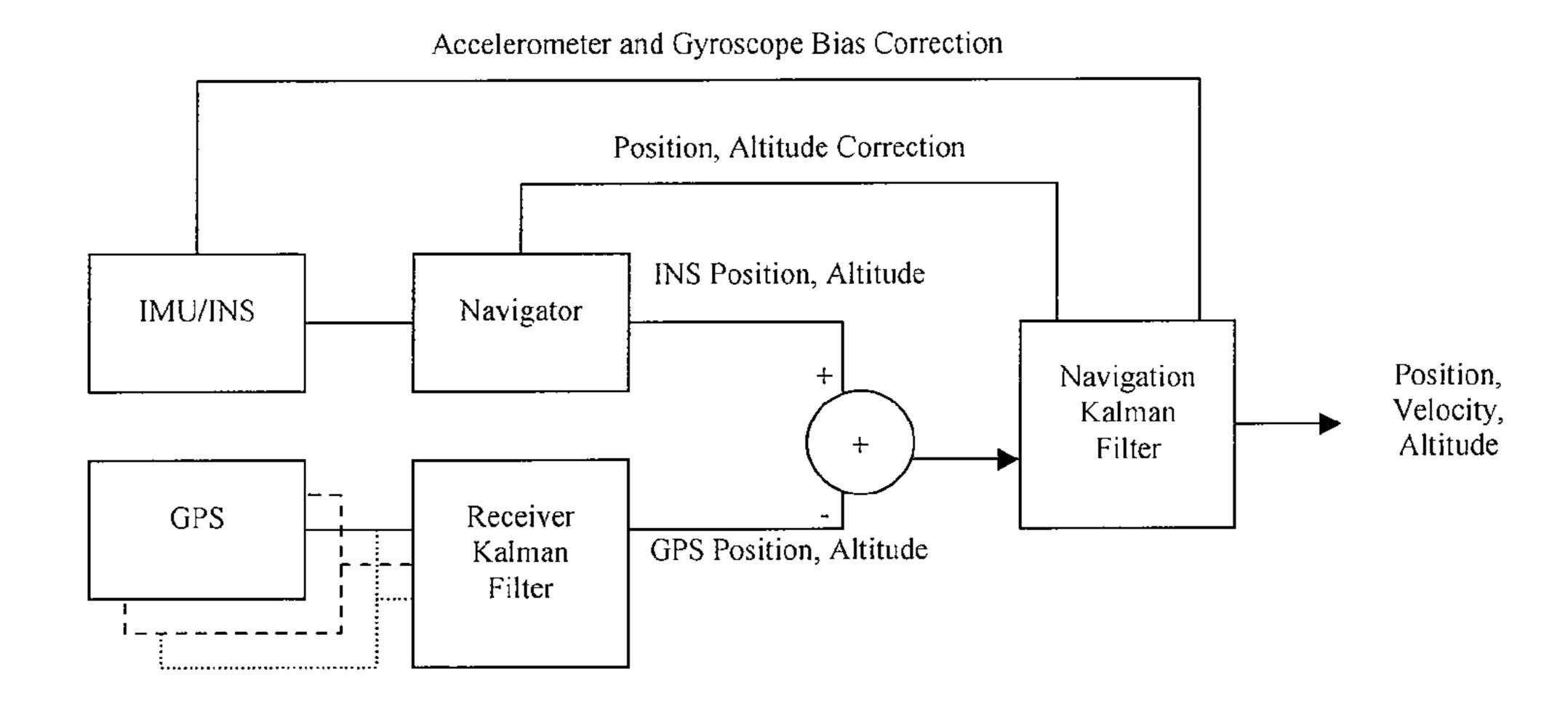
A loosely coupled GPS-IMU/INS system
