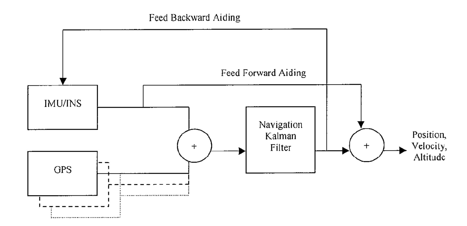
How a Kalman filter can be applied to a combination of GPS and IMU/INS data
