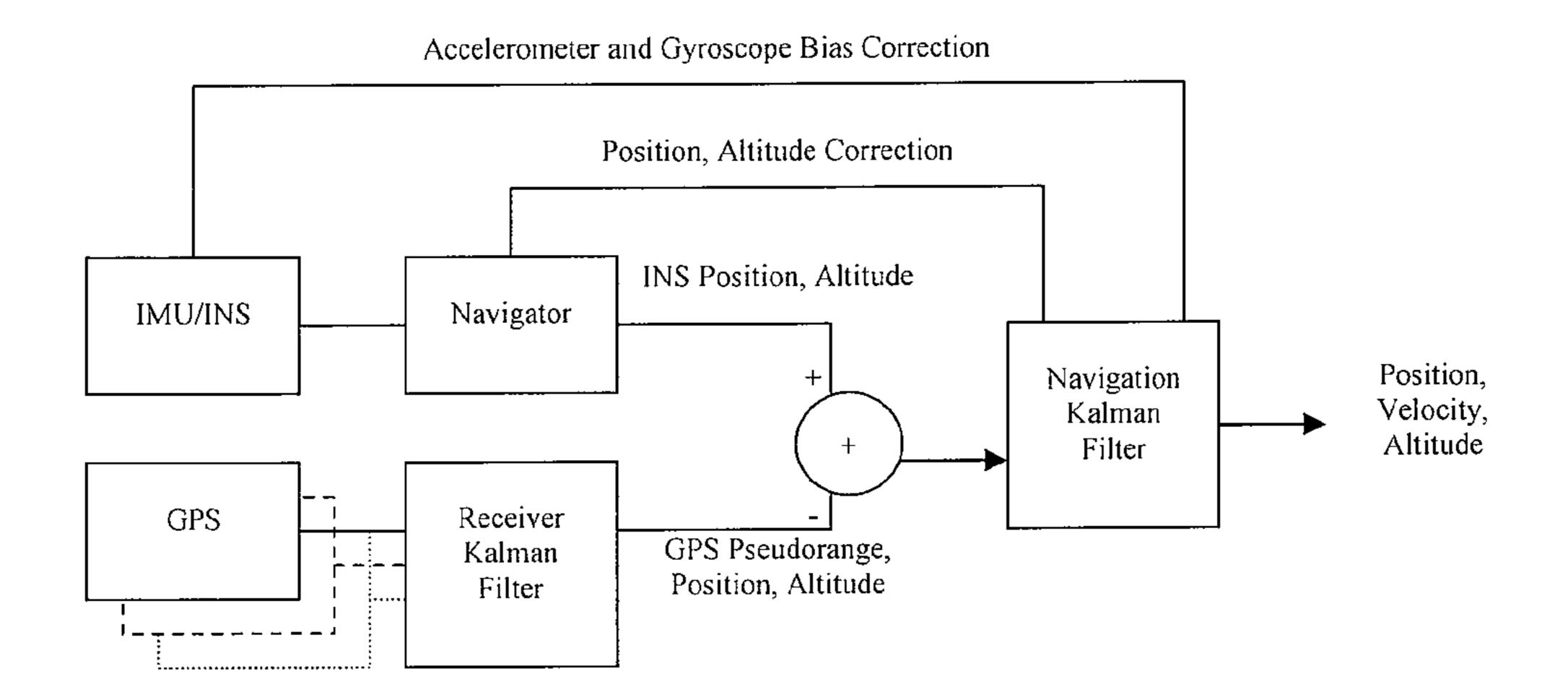
An ultra-tightly coupled GPS-IMU/INS system
