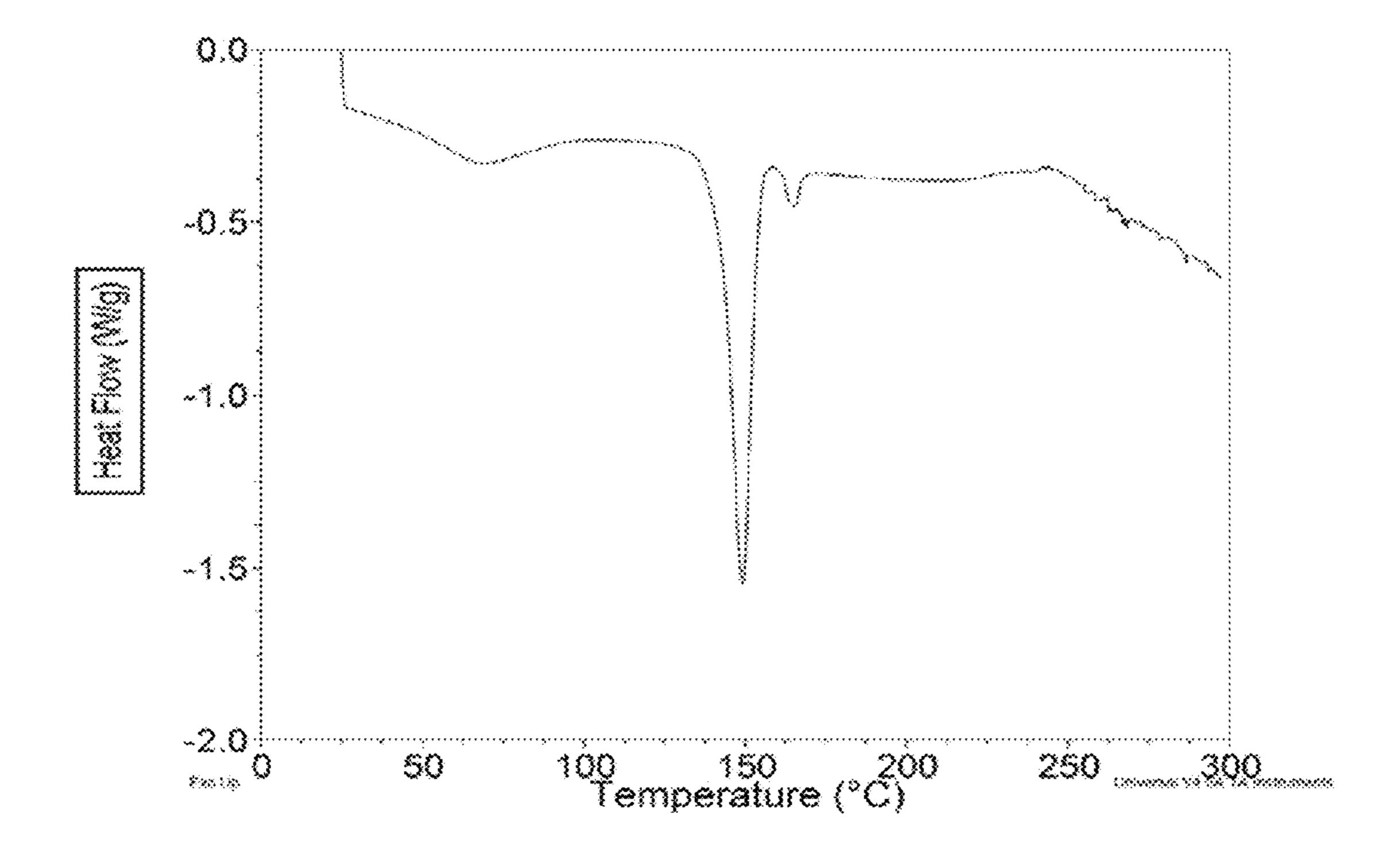
Figure 7: DSC Thermogram 2 - Form B of Compound (I)
