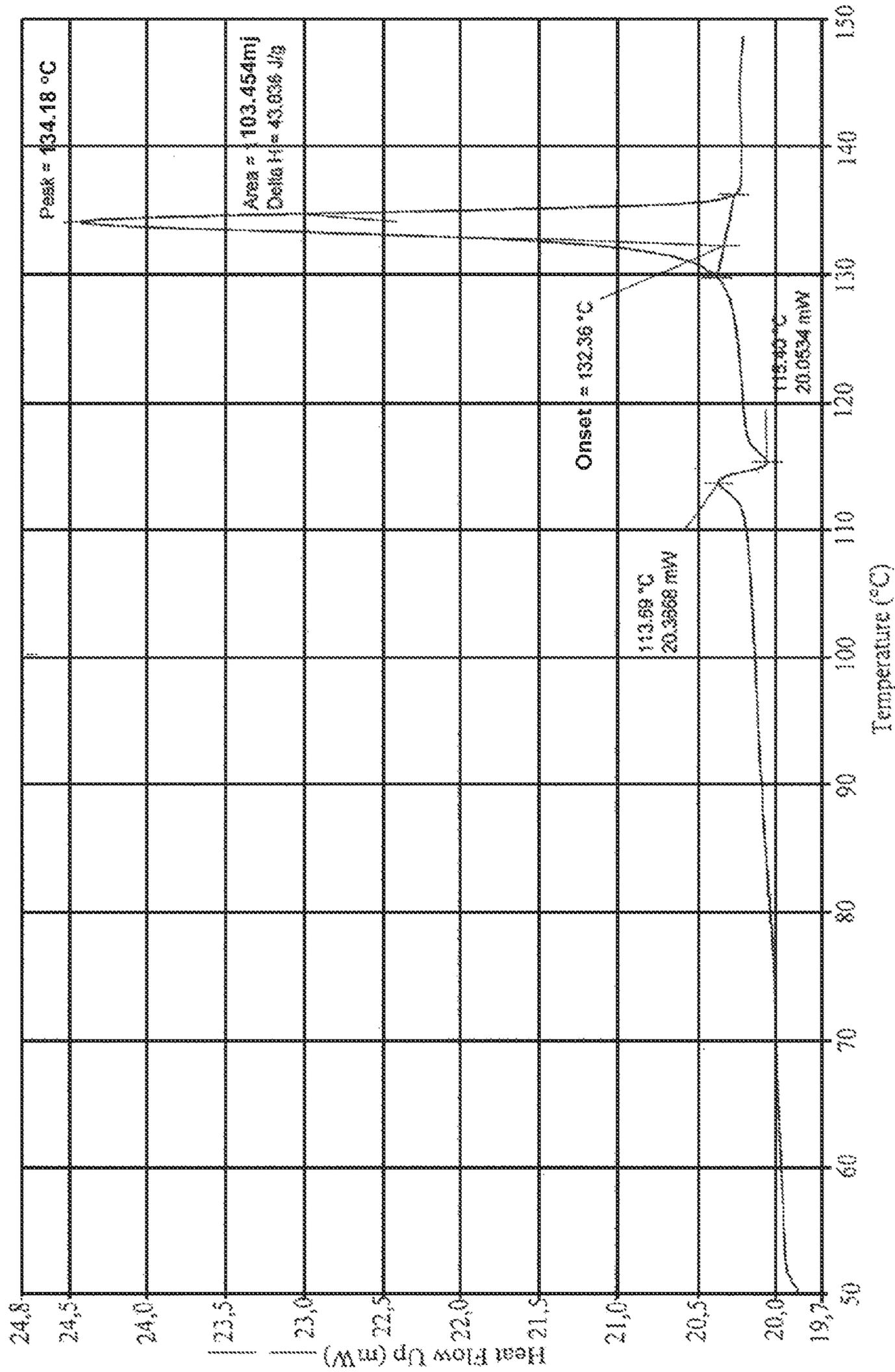
1) Heat from 50.00° to 150.00°C at 5.00°C/min
