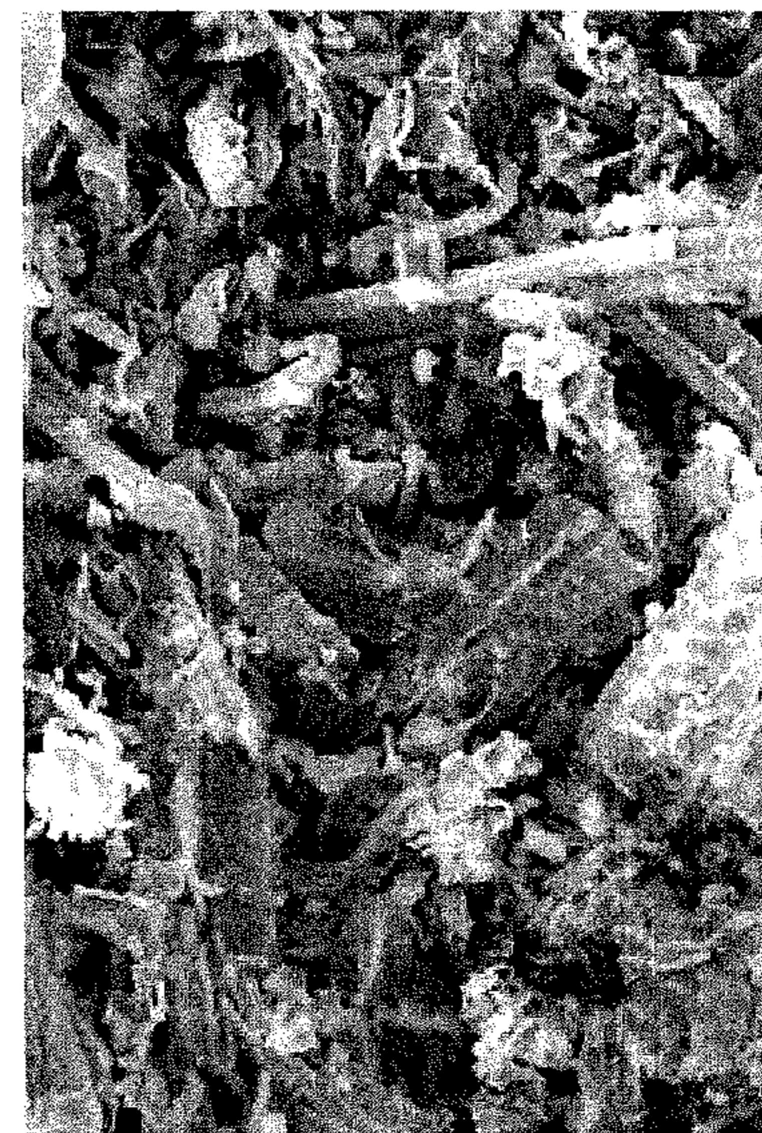
Bio-char, Tube-Furnace, 400°C
