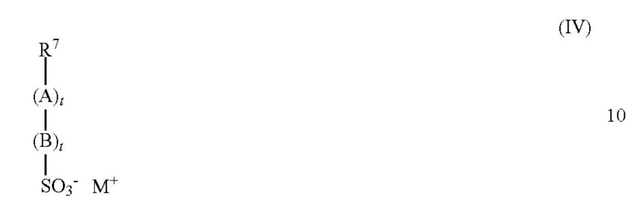
wherein R7 is a group comprising at least one sp2 bond, A is O, N, P, S or an amido or ester linkage, B is a mono- or polycyclic aromatic group or an aliphatic group, each t is independently 0 or 1, and M+ is a cation. In one aspect, R7 is a C2 to C6 alkene. In another aspect, R7 is ethene, butene or propene.
