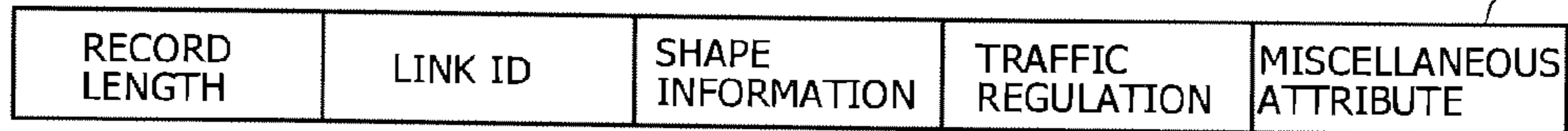
DATA STRUCTURE FOR ONE LINK
