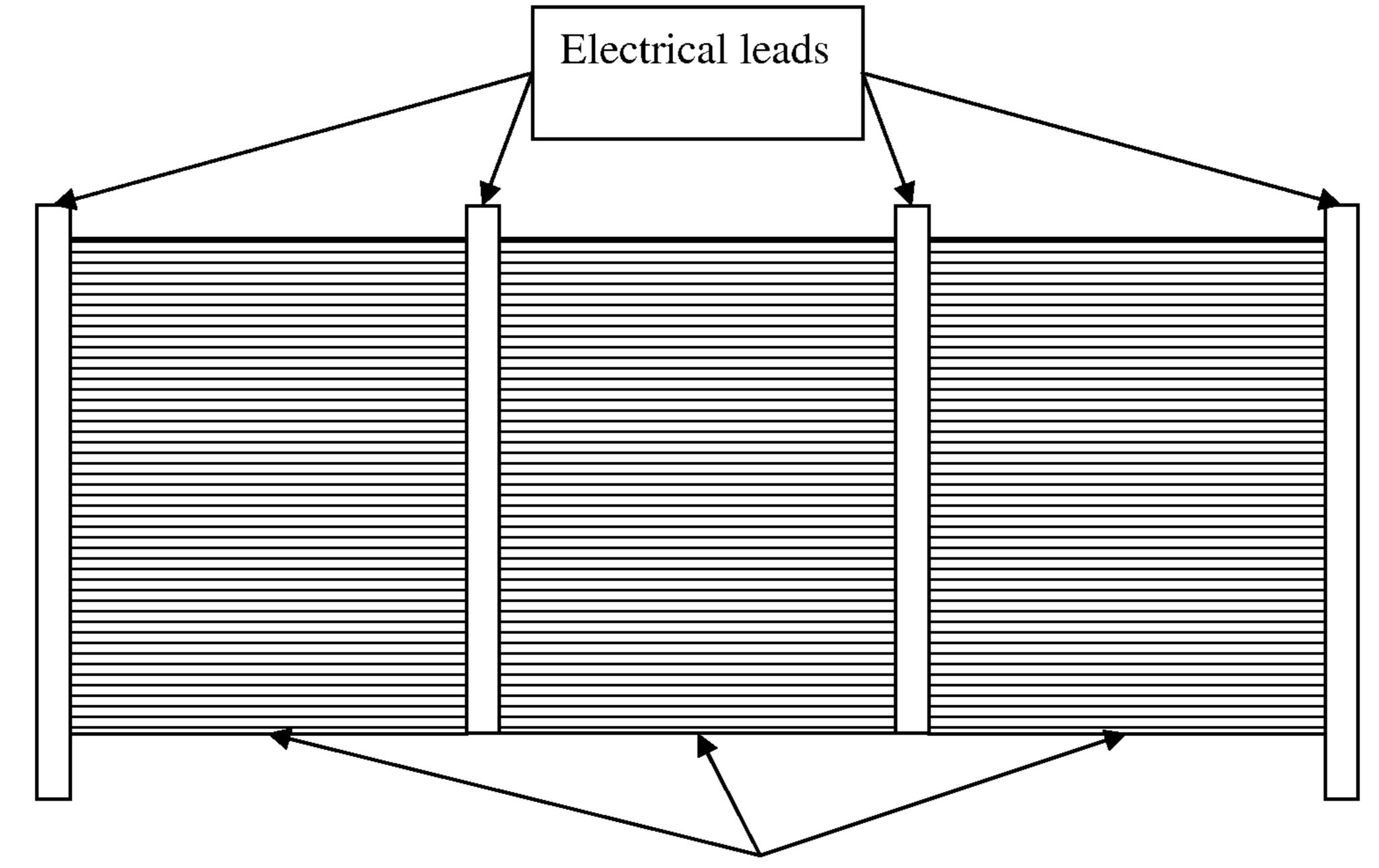
Grooves from embossed polymer filled with carbon nanotubes
