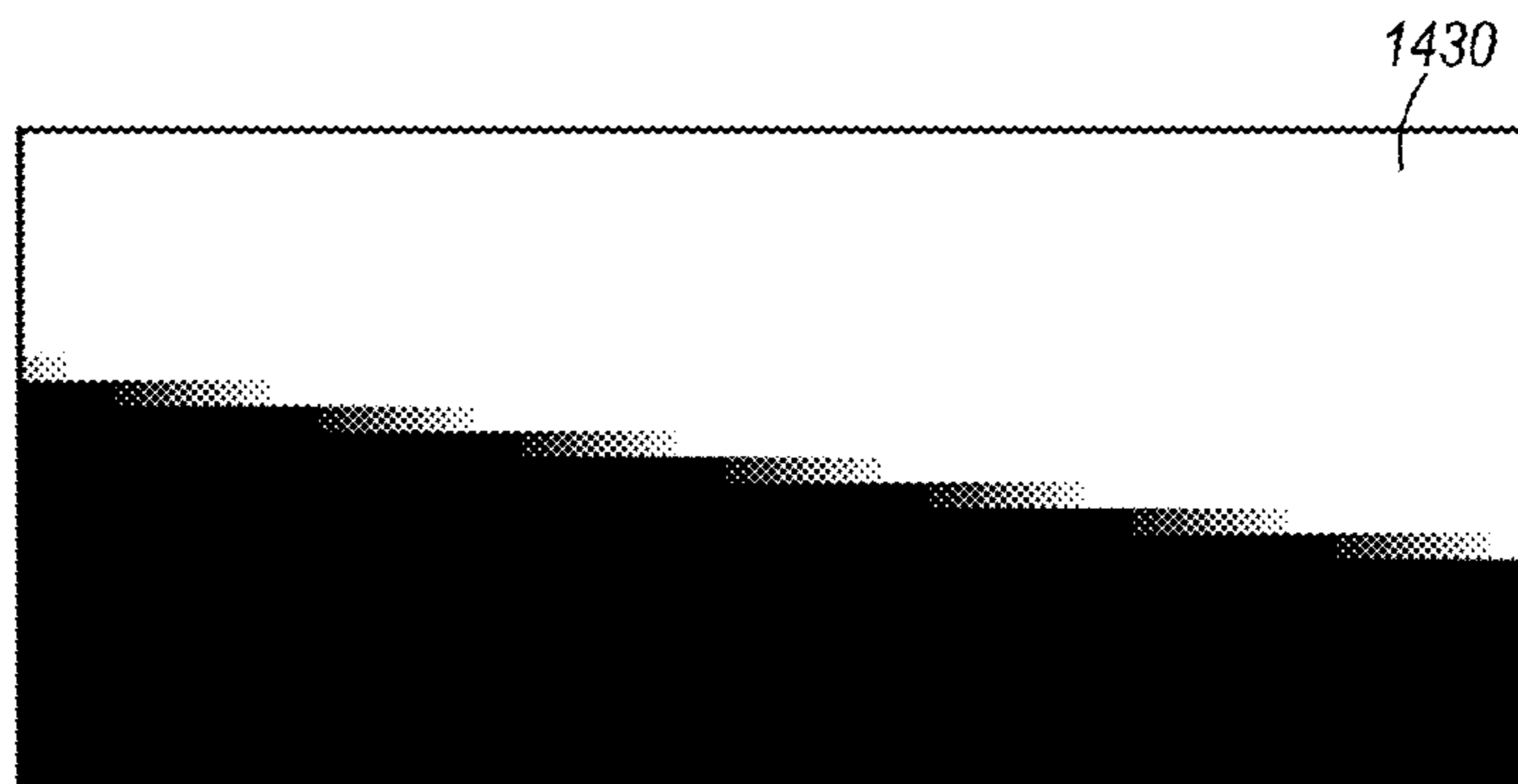
Ideal RGB Sampling of a Black and White 'Slanted Edge' Target
