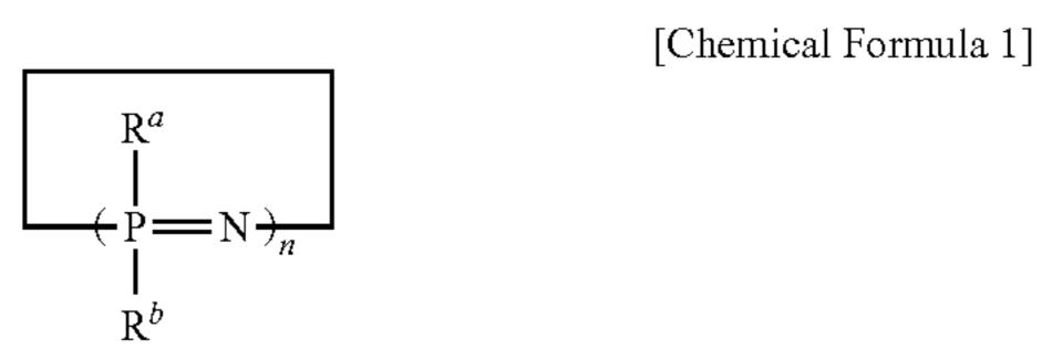
In the above Chemical Formula 1, n is an integer of 3 or 4, and  $R^a$  and  $R^b$  are the same or different and include, for example, F,  $NR_2^1$ , or  $OR_2^1$ , wherein  $R^1$  is a  $C_1$  to  $C_{10}$  alkyl group.
