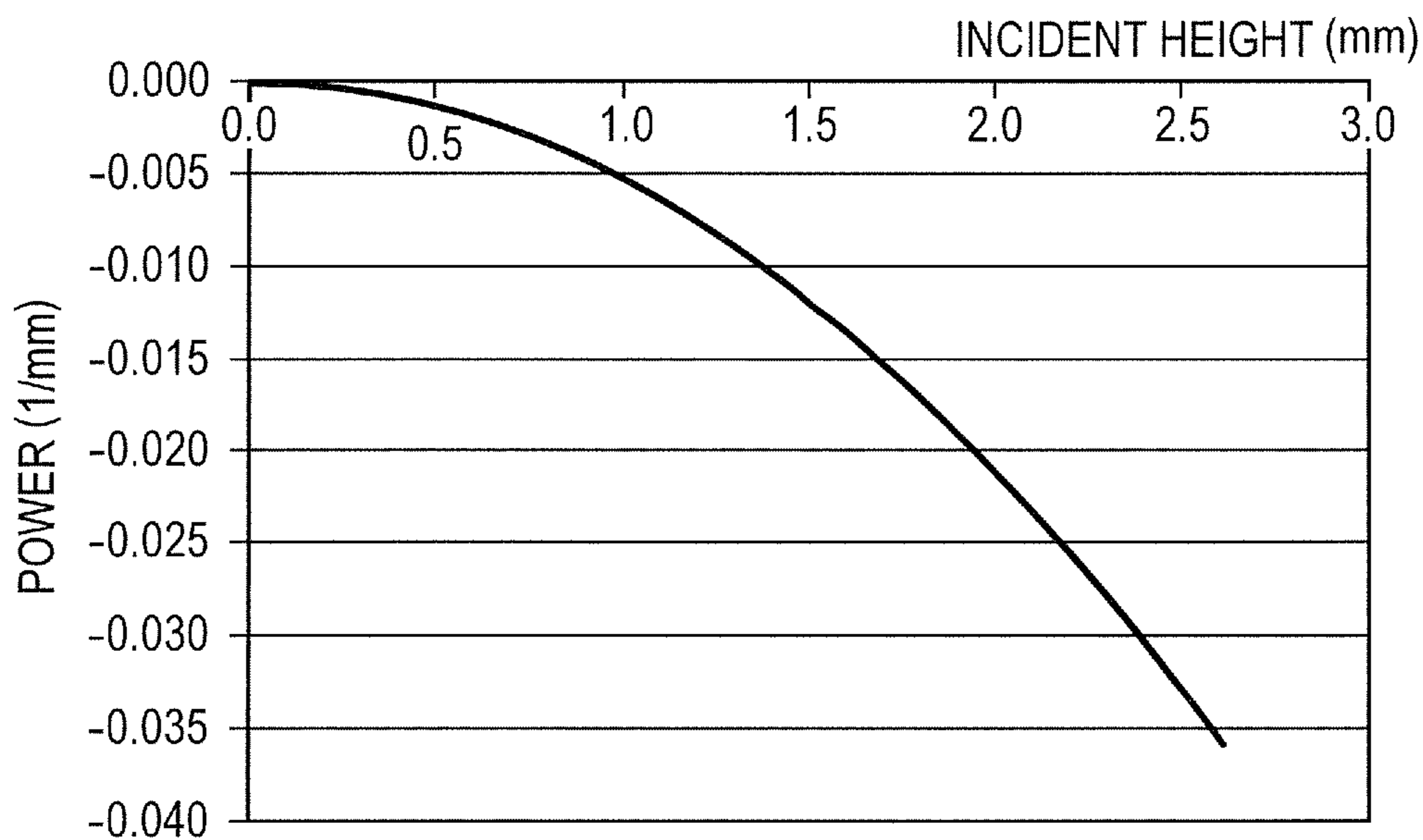
POWER DIFFERENCE DISTRIBUTION DUE TO PHASE DIFFERENCE
