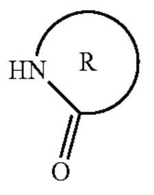
where R represents a  $C_3$  to  $C_{12}$  substituted or unsubstituted cyclic hydrocarbon chain. The polymerization of these lactam monomers involves the opening of the cyclic hydrocarbon chain to make a linear chain with reactive carbonyl and amine groups separated by a  $-(CH_2)_n$  hydrocarbon group.
