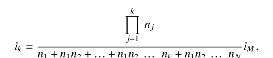
in which  $i_k$  is the branch current in the k-th branch,  $n_k$  is a turn ratio of the k-th transformer unit and  $i_M$  is the input current to be distributed.
