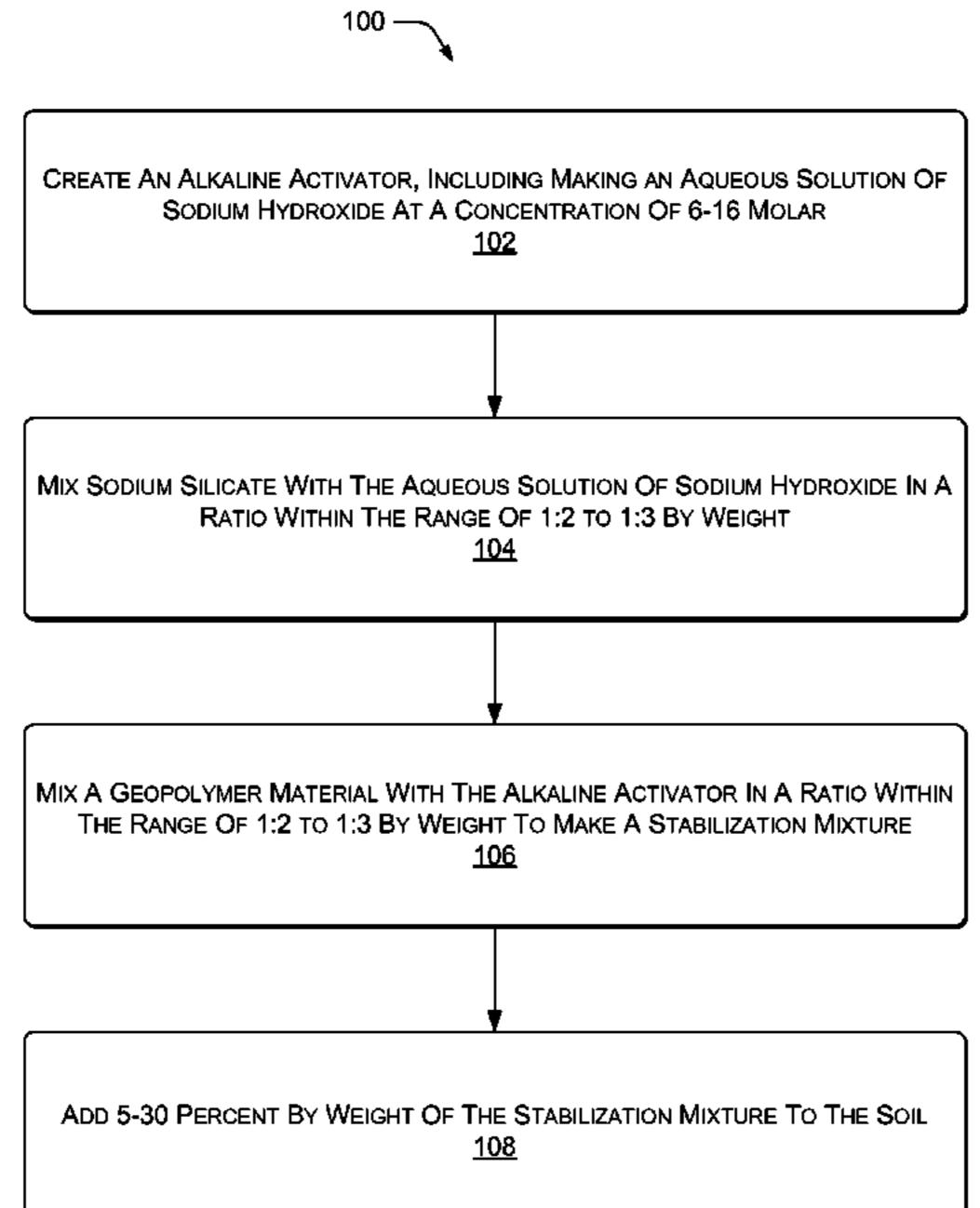
CREATE AN ALKALINE ACTIVATOR, INCLUDING MAKING AN AQUEOUS SOLUTION OF SODIUM HYDROXIDE AT A CONCENTRATION OF 6-16 MOLAR 102
