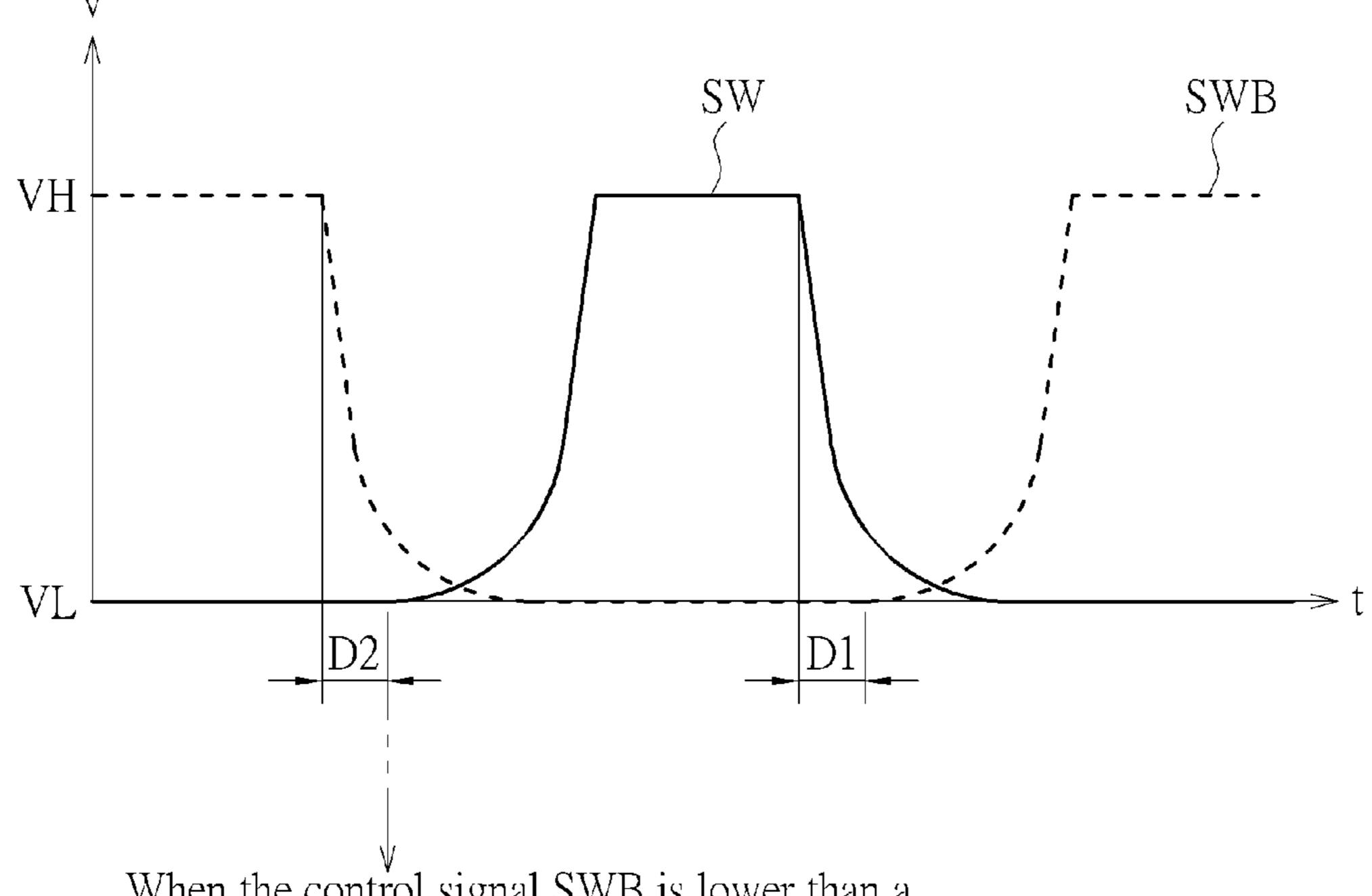
When the control signal SWB is lower than a predetermined voltage, the control signal SW starts to switch from the low voltage (VL) to the high voltage (VH)
