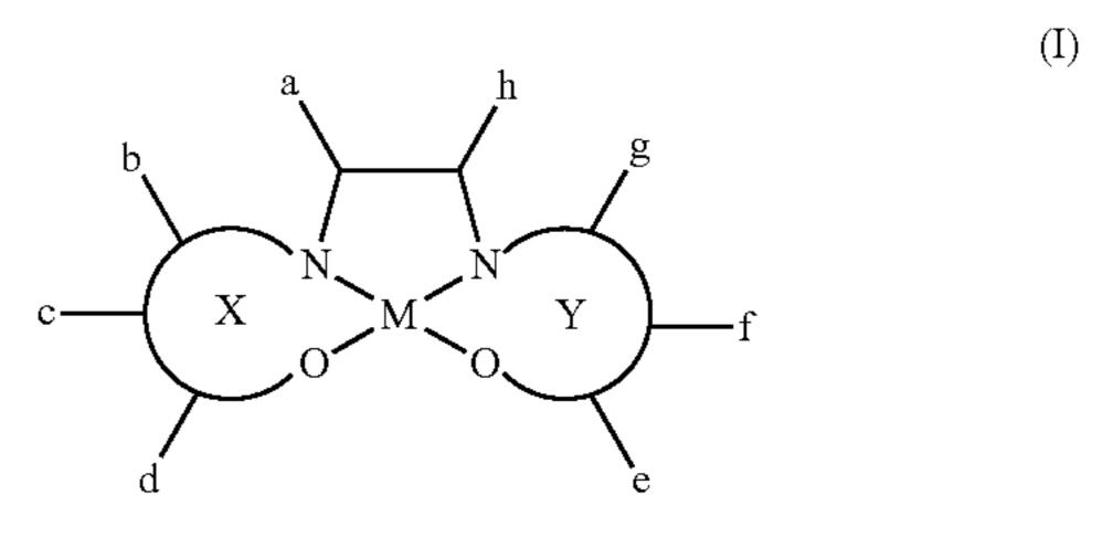
Each of X and Y is a five-membered ring structure including a coordinate bond between N and M, or its six-membered ring structure, wherein M is a bivalent metal3
