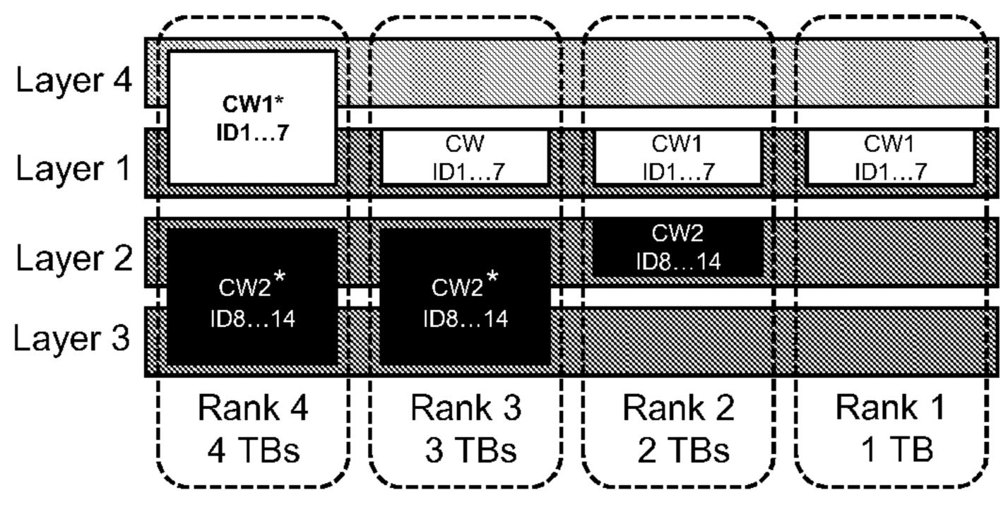
\* A codeword contains two transport blocks and is interleaved across two layers
