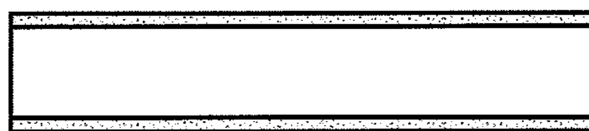
(A) GROW \text{SiO}_2 LAYER BY THERMAL OXIDATION ON Si WAFER
