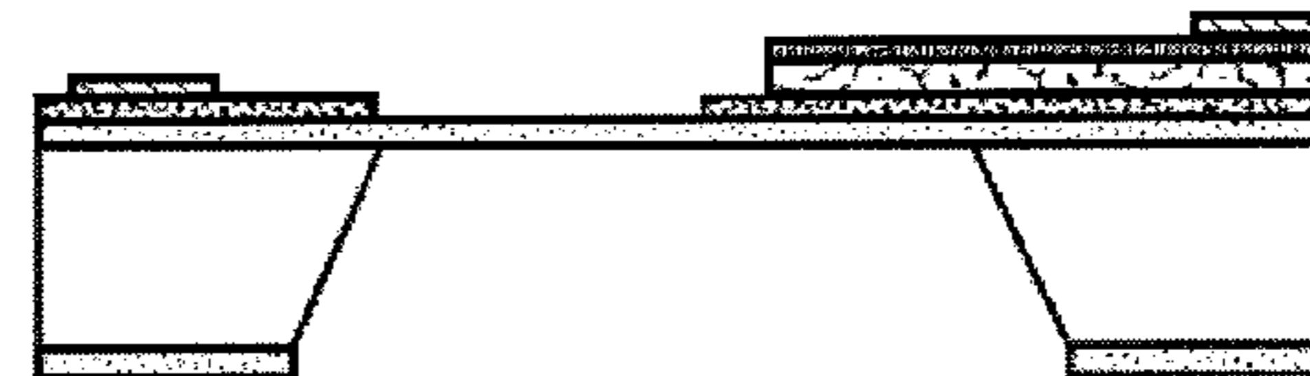
(H) ETCH Si FROM BACK SIDE BY KOH
