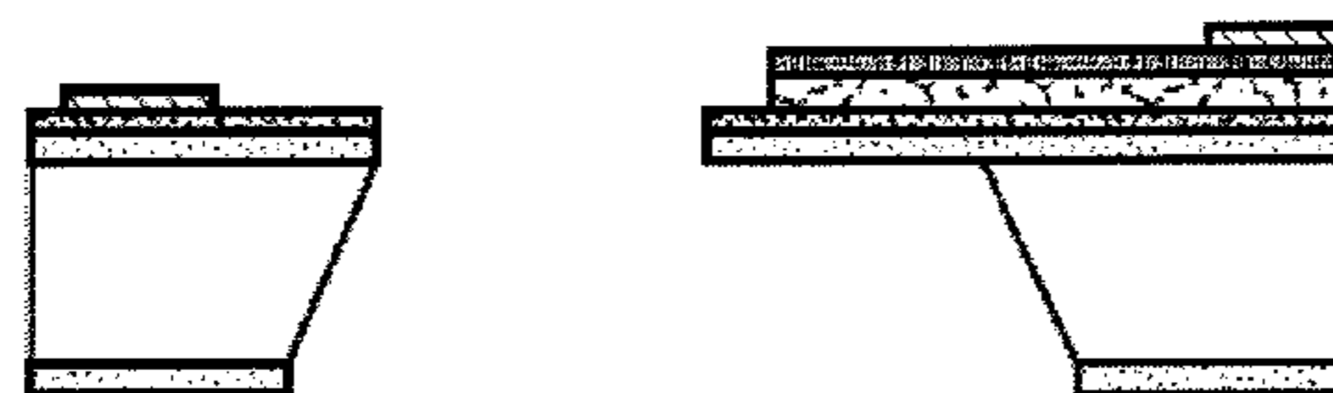
(I) ETCH \text{SiO}_2 FROM THE FRONT SIDE BY RIE TO RELEASE CANTILEVER
