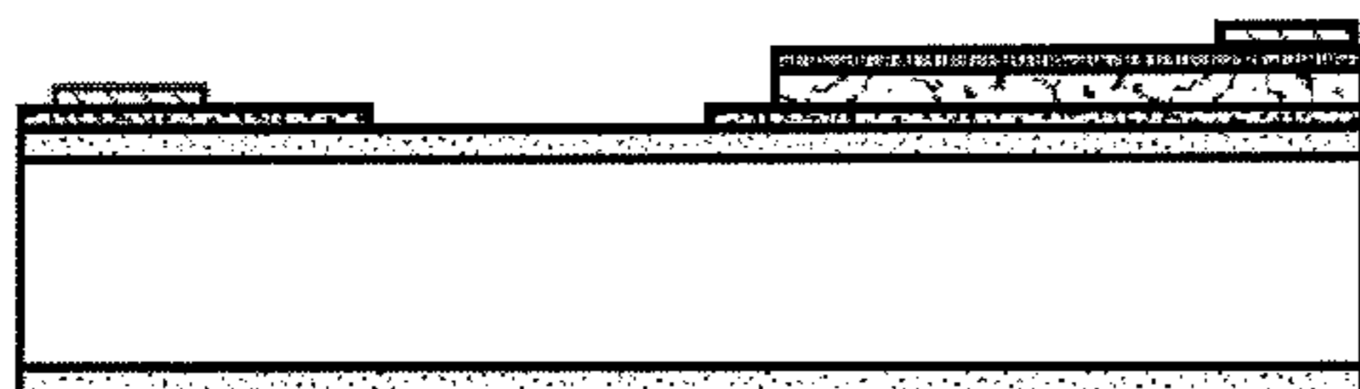
(G) DEPOSIT AND PATTERN Au BONDING PAD ON ELECTRODE
