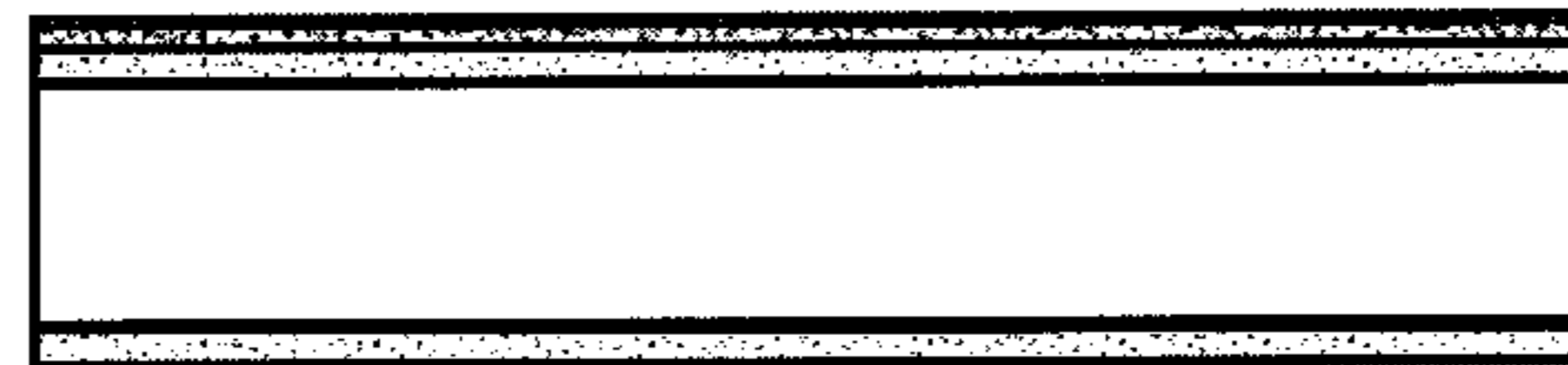
(B) DEPOSIT TiO x /Pt BOTTOM ELECTRODE BY REACTIVE SPUTTERING
