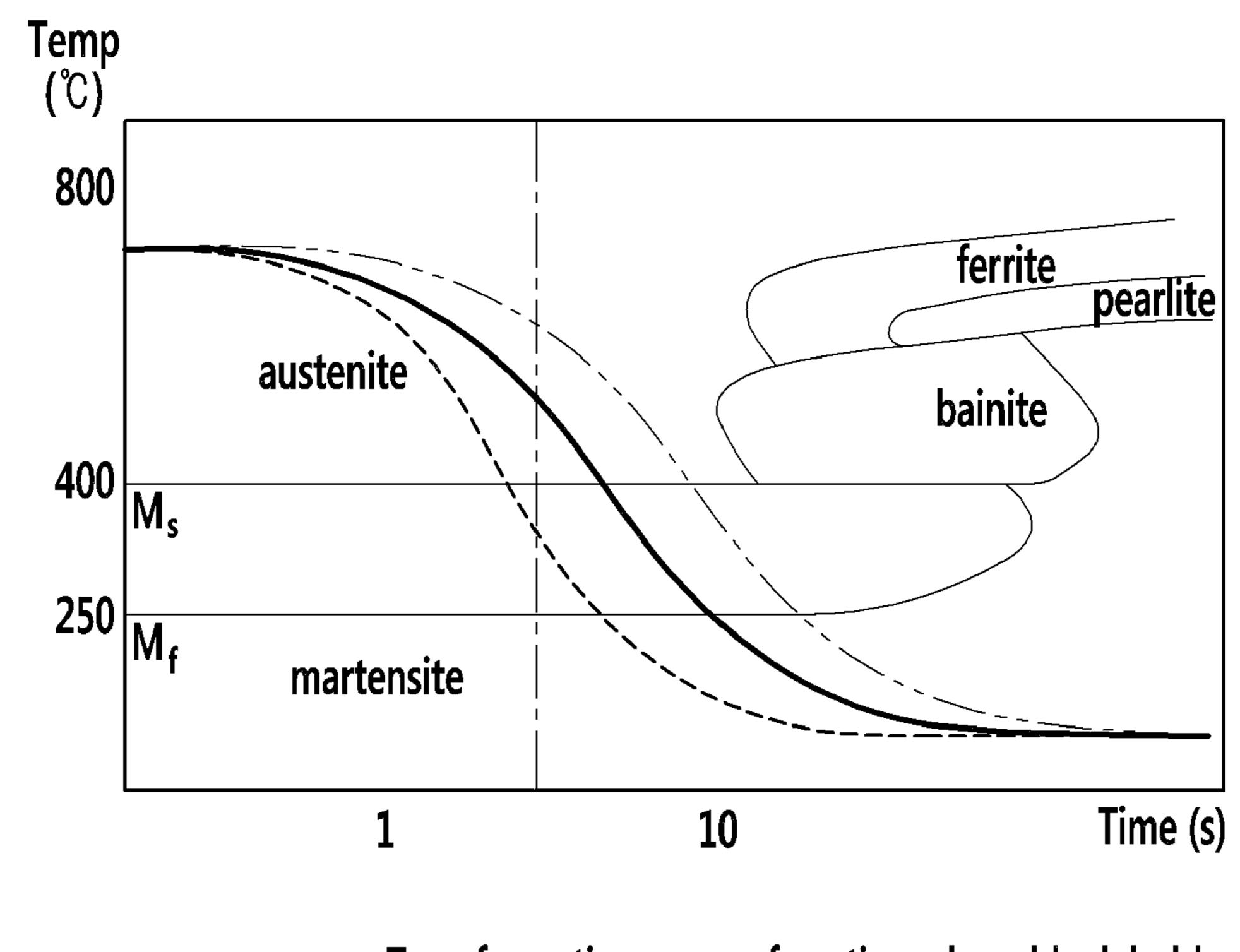
Transformation curve of portion where blank holder and blank are in contact (a)
