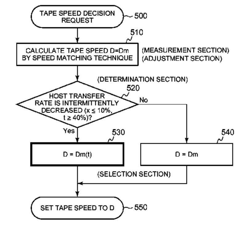
NOTE: - DRIVE TRANSFER RATE (DATA TRANSFER RATE BETWEEN BUFFER AND TAPE): DEPENDING ON TAPE SPEED SPEED MATCHING TECHNIQUE: ADJUST TAPE SPEED TO MATCH DRIVE TRANSFER RATE TO HOST TRANSFER RATE IN ORDER TO AVOID BACK HITCH CAUSED WHEN BUFFER IS FILLED UP WITH DATA (UPON READ FROM HOST) AND WHEN BUFFER IS EMPTIED OF DATA (UPON WRITE FROM HOST)
