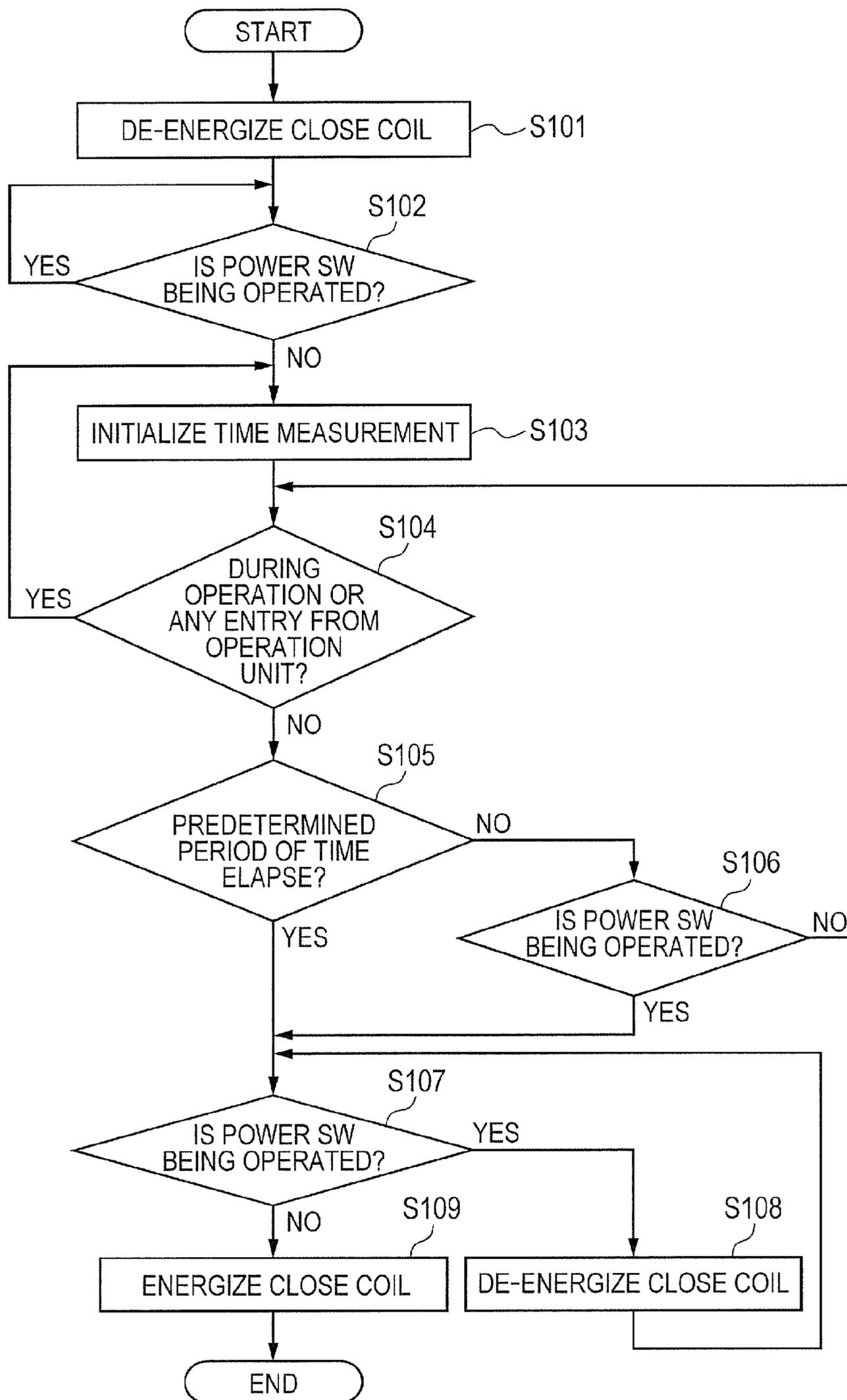
**1****POWER SUPPLY CONTROL FOR AN IMAGE FORMING APPARATUS**
