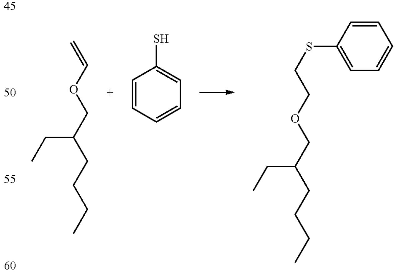
7.0 grams (44.79 mmo, MW: 156.27) 2-ethylhexylvinylether, 5.93 grams (53.75 mmol, MW: 110.18) thiophenol and 0.368 grams (2.240 mmol, MW: 164.21) 2,2'-azobis(2-methylpropionitrile) (AIBN) were charged in a 25 milliliter thick sealed glass reactor. After addition, the reaction mixture was stirred for 24 hours at 115° C. The reaction was then
