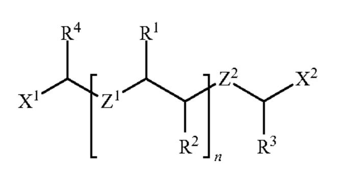
wherein X¹ and X², Z¹ and Z², R¹, R², R³, and R⁴, and n are as defined herein, a polyhydroxy aromatic compound, a polyvinyl alcohol, and water, wherein the polishing composition has a pH of about 1 to about 4.5. The invention further provides a method of chemically-mechanically polishing a substrate with the inventive chemical-mechanical polishing composition. Typically, the substrate contains silicon oxide, silicon nitride, and/ or polysilicon.
