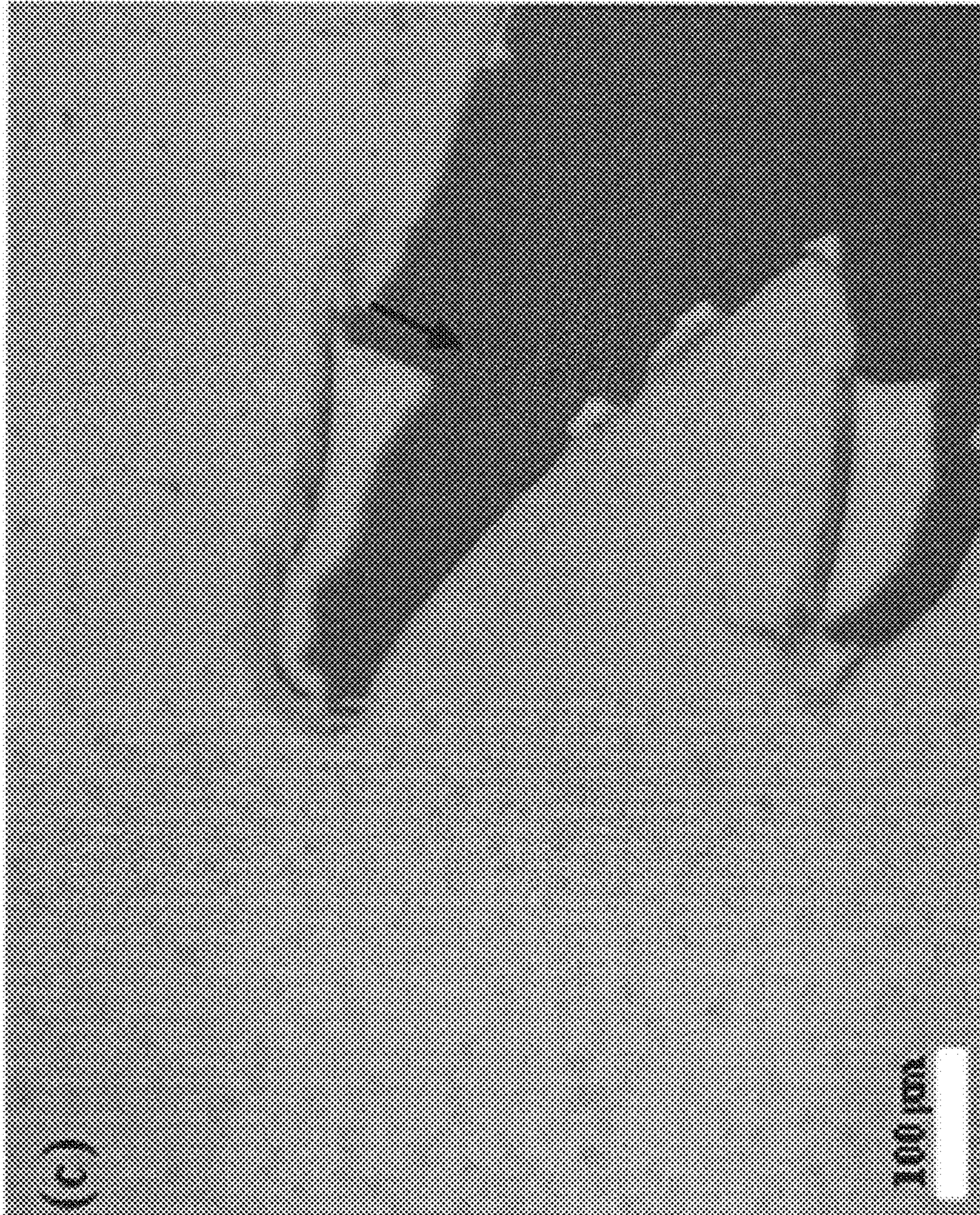
40 nm ALD Al 2 O 3 film passivation in LB media after 2 days
