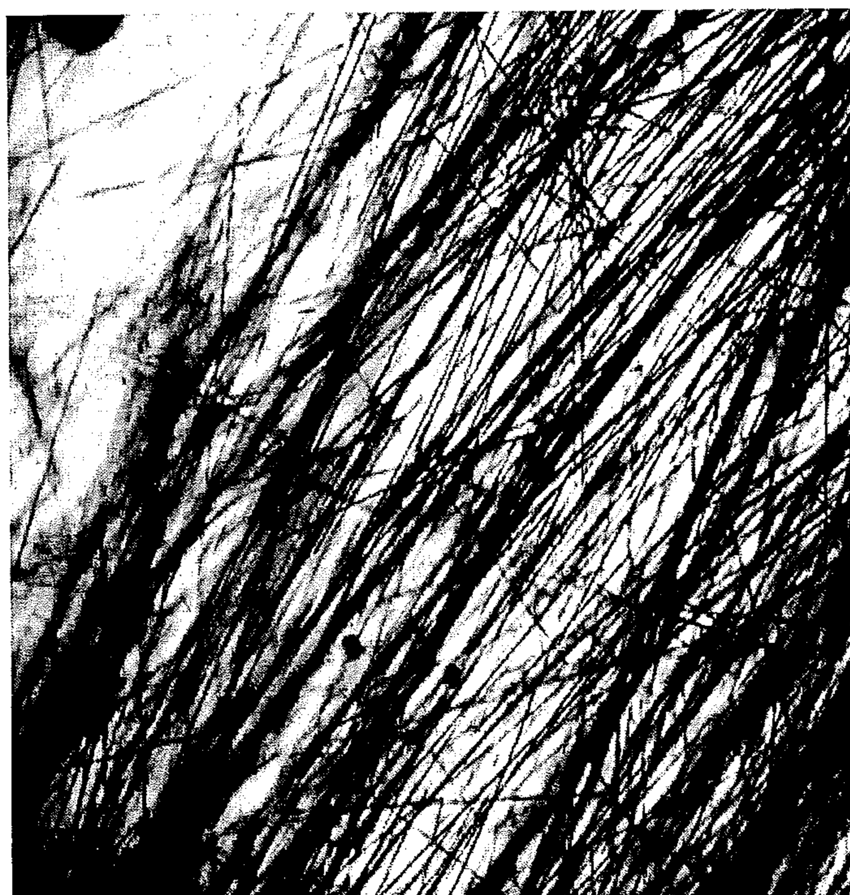
FIGURE 3 FIBRE ORIENTATION WITHIN THE CARDED SLIVER
