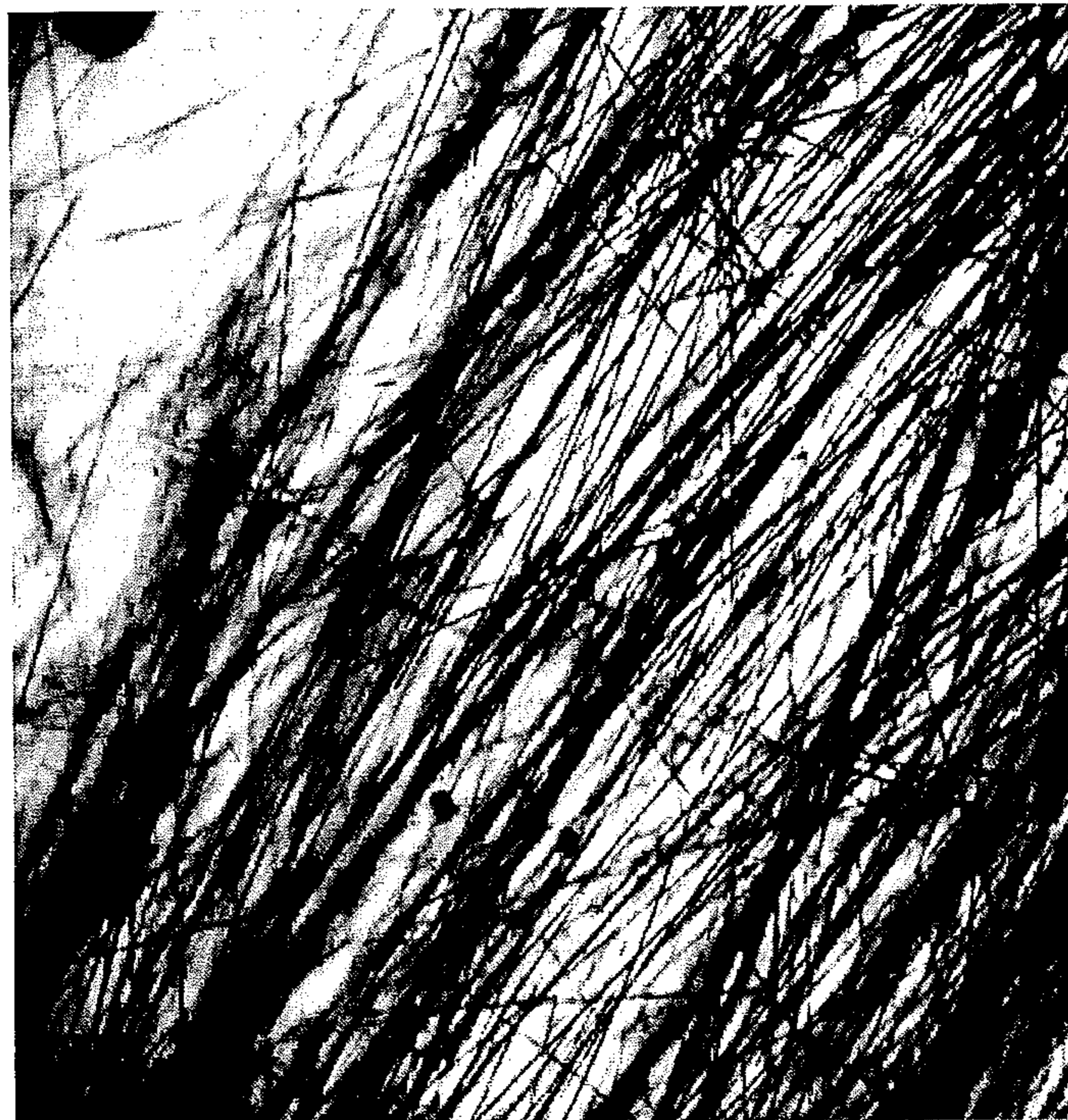
FIGURE 3 FIBRE ORIENTATION WITHIN THE CARDED SLIVER
