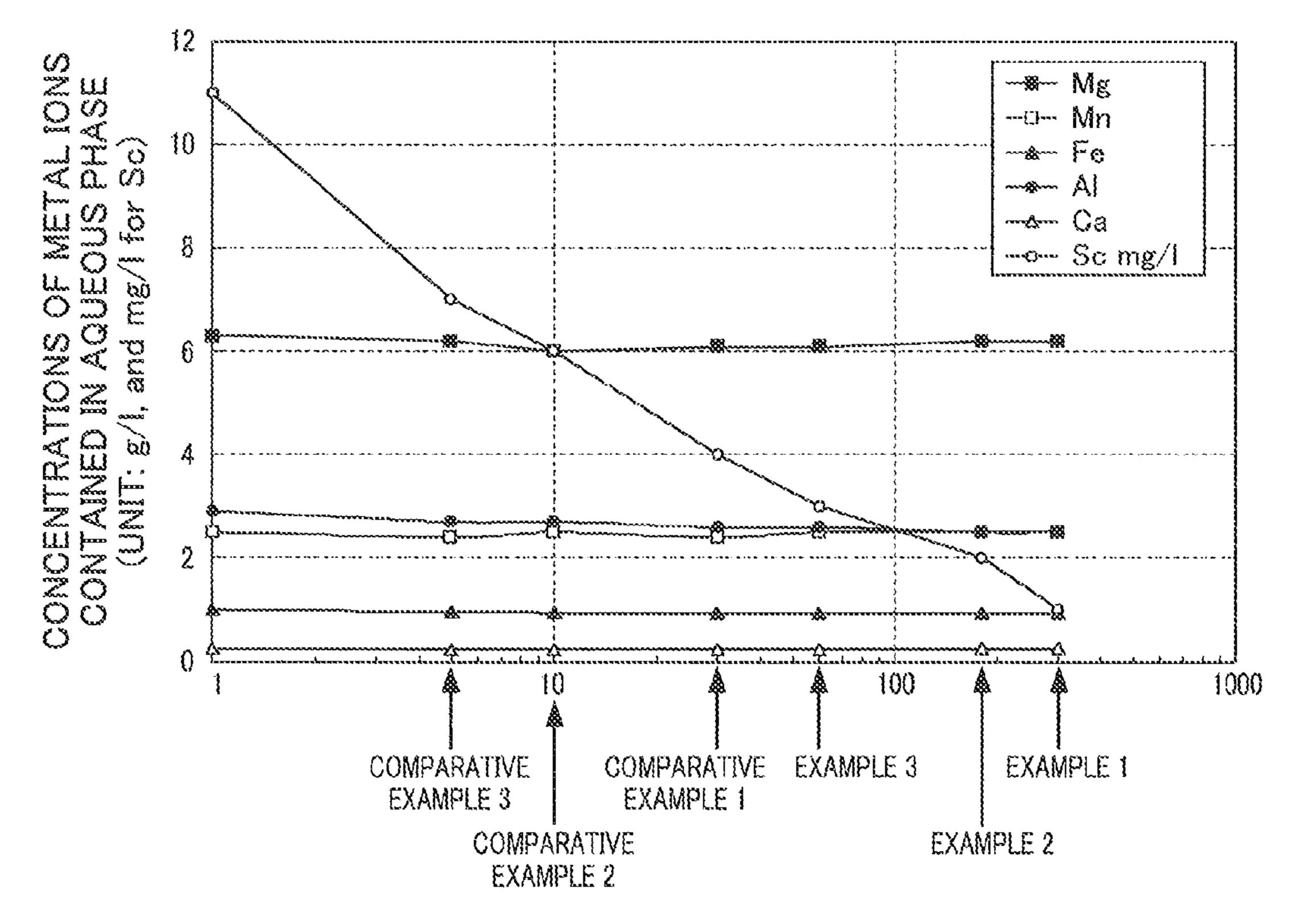
CONTACT TIME OF ACID SOLUTION AND SCANDIUM RECOVERING RESIN (min.)
