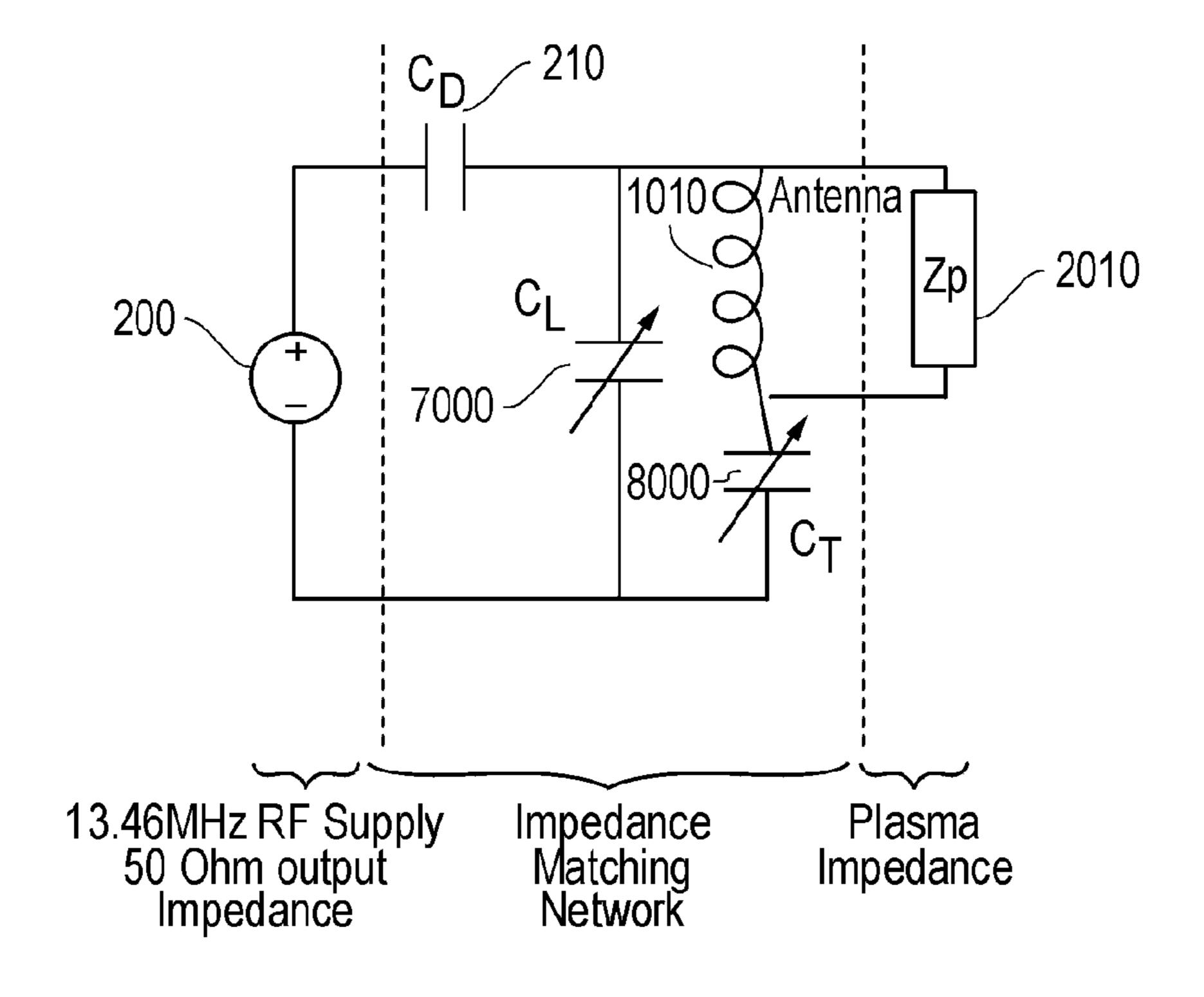
C<sub>D</sub>=200pF, C<sub>L</sub>=92pF,C<sub>T</sub>=216pf, Phase shift across antenna=0° C<sub>D</sub>=50pF, C<sub>L</sub>=330pF,C<sub>T</sub>=340pf, Phase shift across antenna=180°
