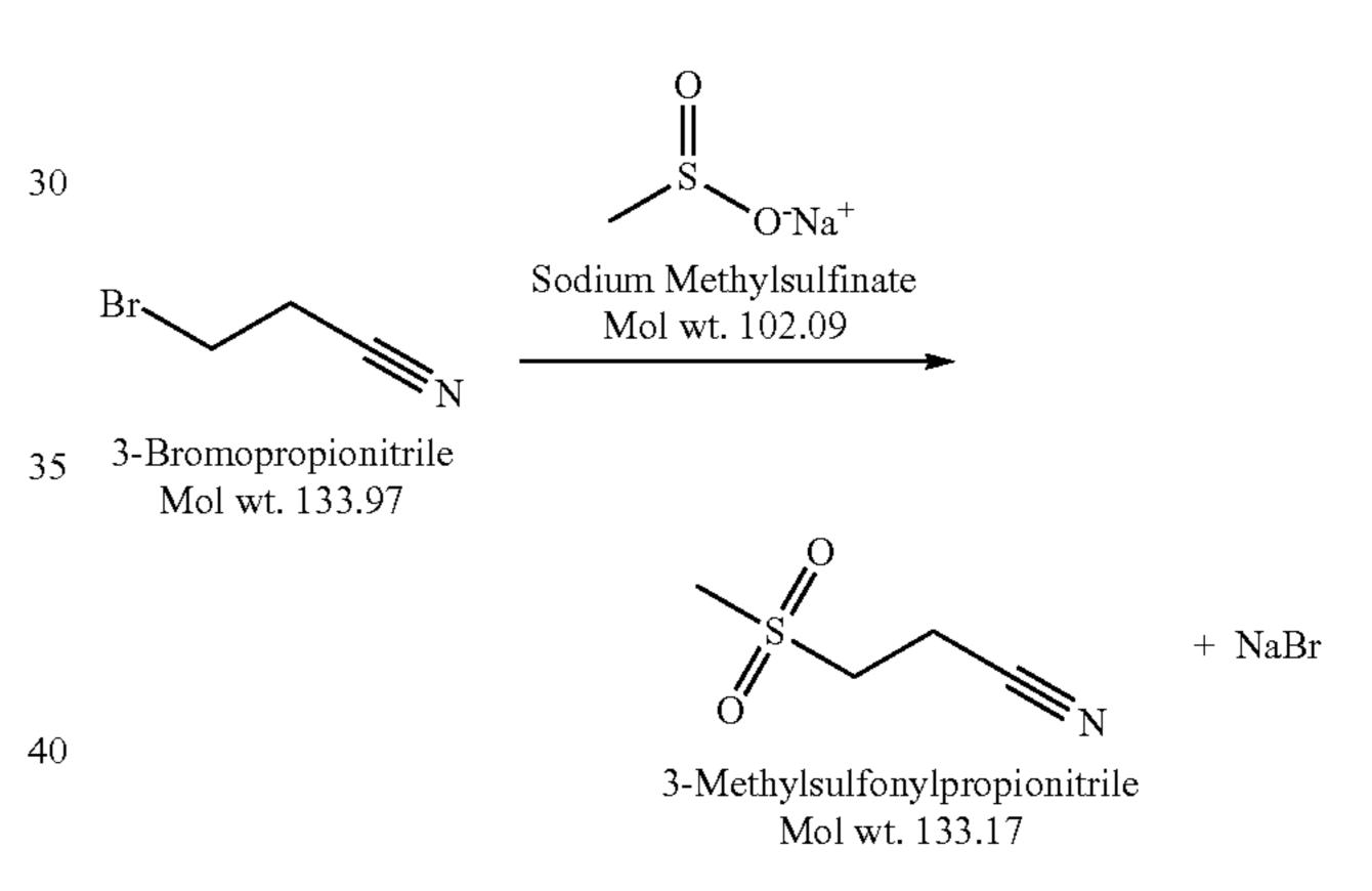
An organic solvent is used in the reaction to facilitate the alkylation and enable isolation of a crude product filter cake (mixture of 3-methylpropionitrile and sodium bromide NaBr). Examples of suitable organic solvents include ethanol, methanol, propanol, isopropanol, butanol, or a mixture thereof. Preferred organic solvent is ethanol, or a mixture of alcoholic solvents containing ethanol (e.g., ethanol/methanol/isopropanol at 90/5/5).
