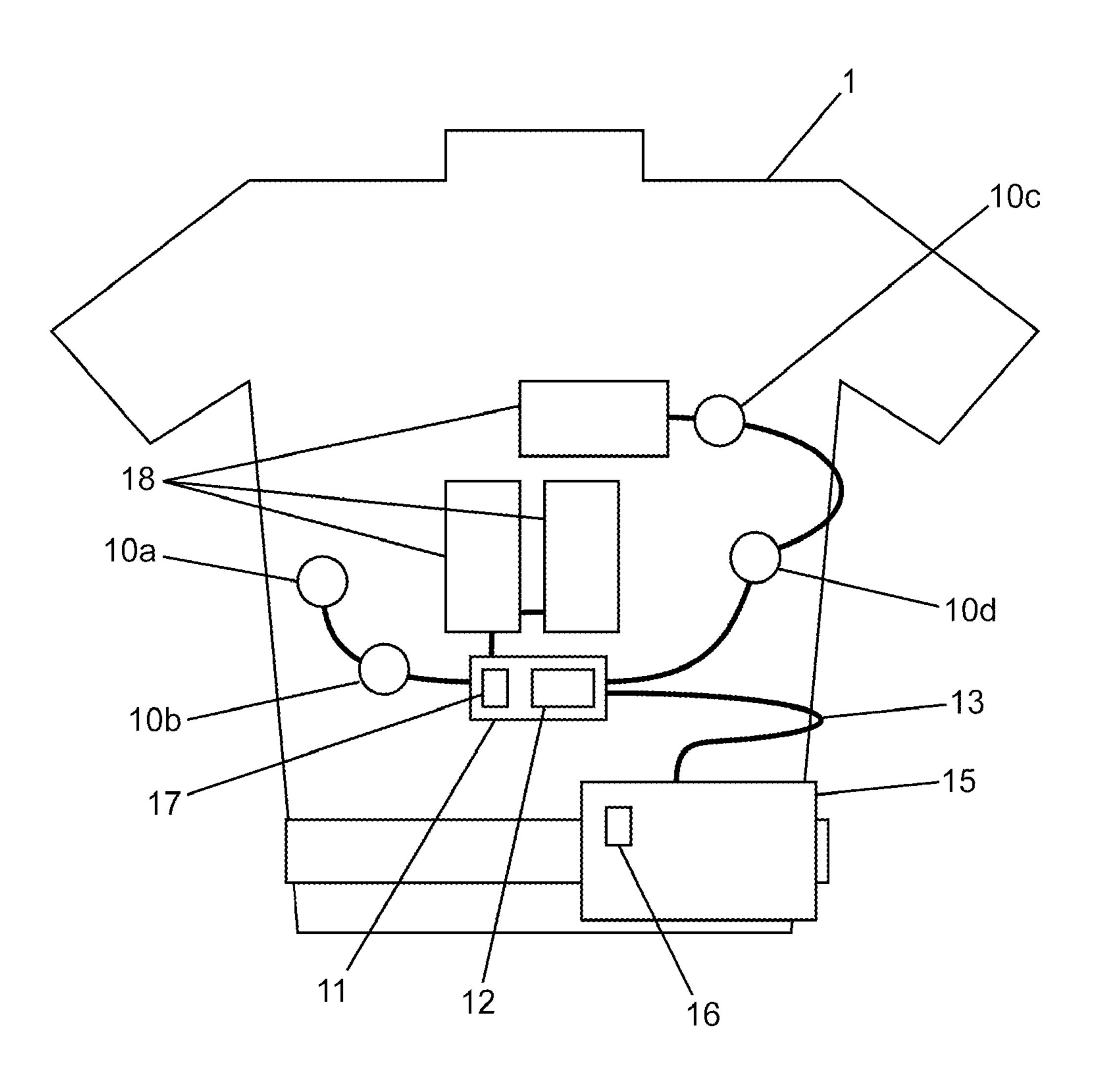
Figure 2: System diagram with accelerometers
