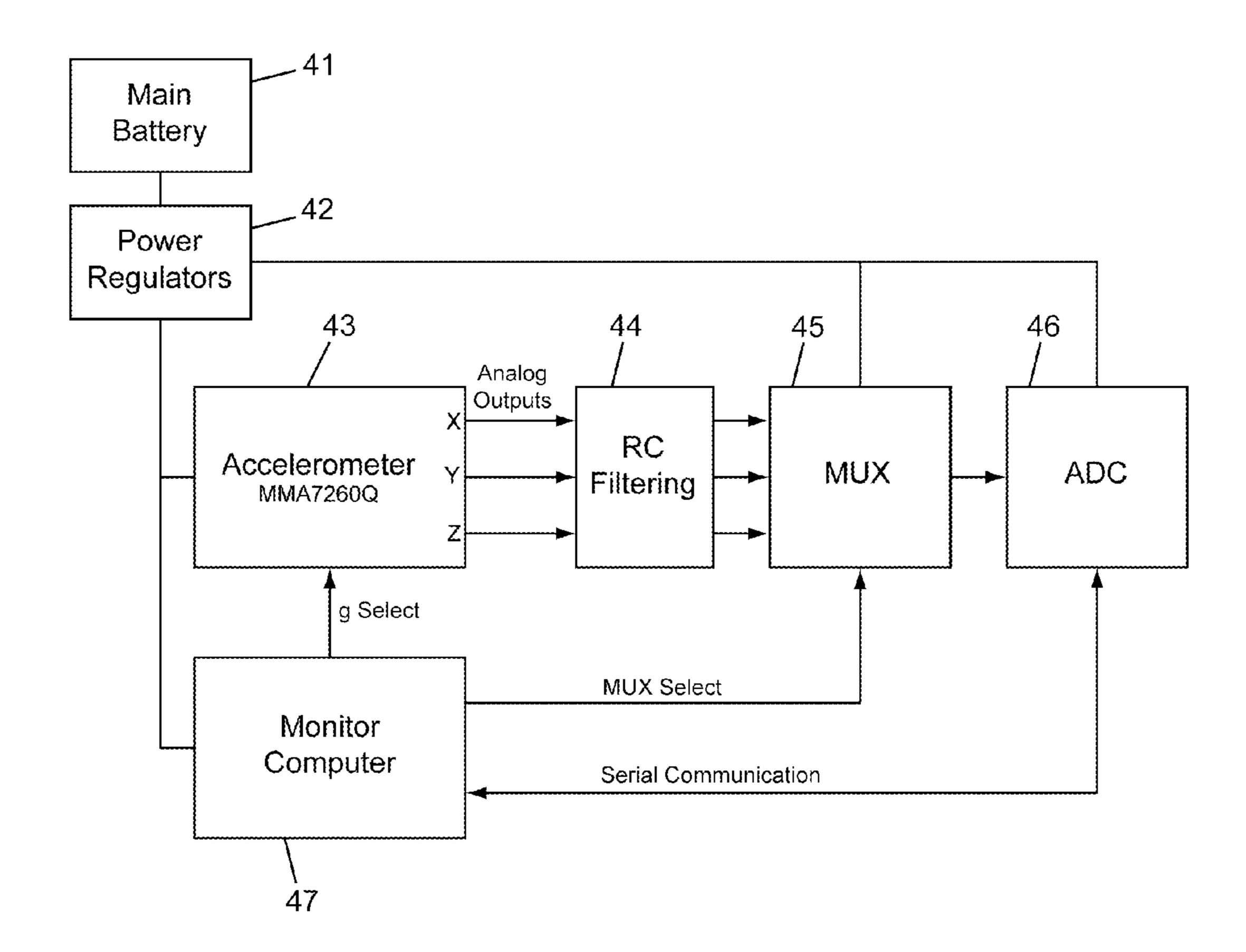
Figure 4: Belt Node Accelerometer
