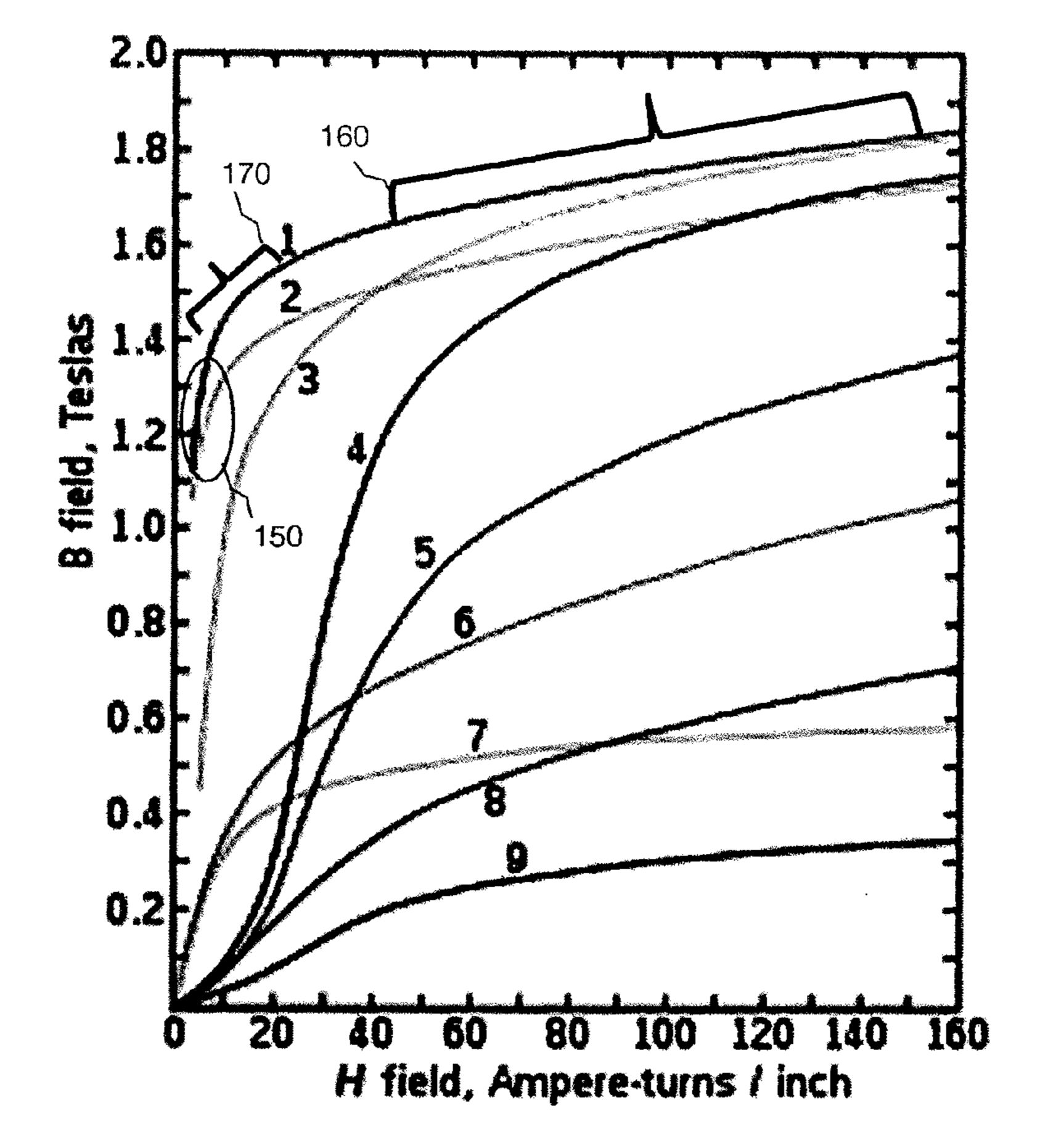
Magnetization curves of 9 ferromagnetic materials, showing saturation.
