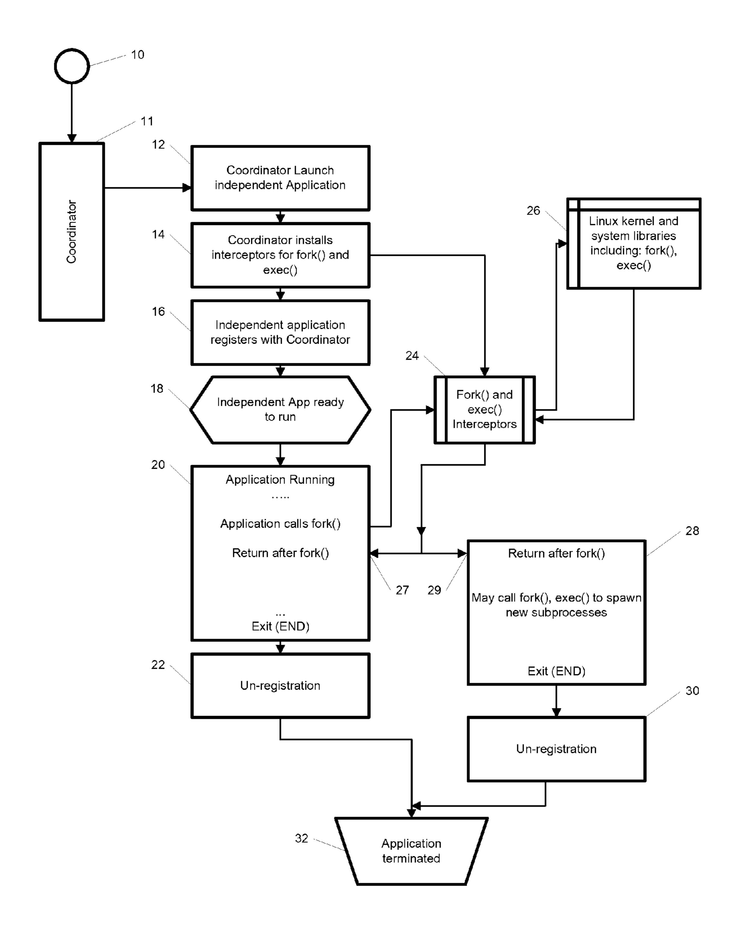
Fig. 1 – Core operation of fork()
