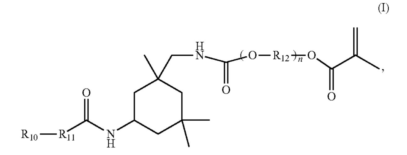
In formula (I),  $R_{10}$  is fluoroalkyl group ( $C_xF_yH_z$ , wherein x is an integer of 2-20, y is an integer of 5-30, and y+z=2x-1),  $R_{11}$  is oxygen, nitrogen or sulfur;  $R_{12}$  is  $C_1$ - $C_3$  alkylene; n is an integer of 3-40.
