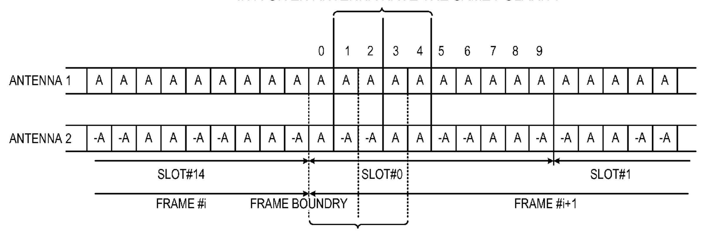
PAIRS NOT TO BE SELECTED: SOFT PILOT SYMBOLS IN A GIVEN ANTENNA HAVE DIFFERENT POLARITIES
