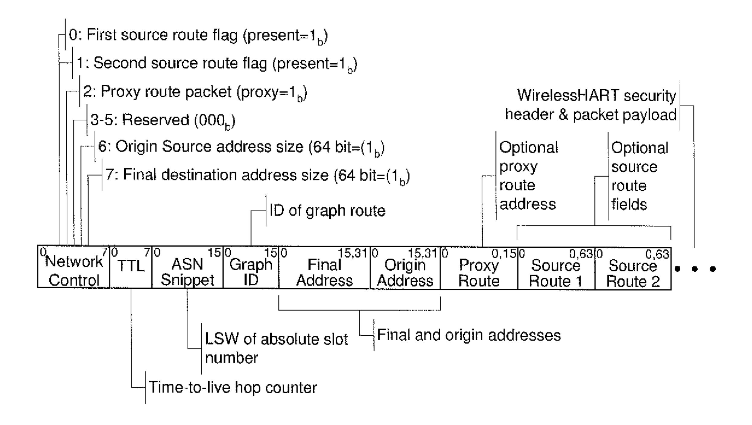
FIG. 7 WirelessHART Network Header
