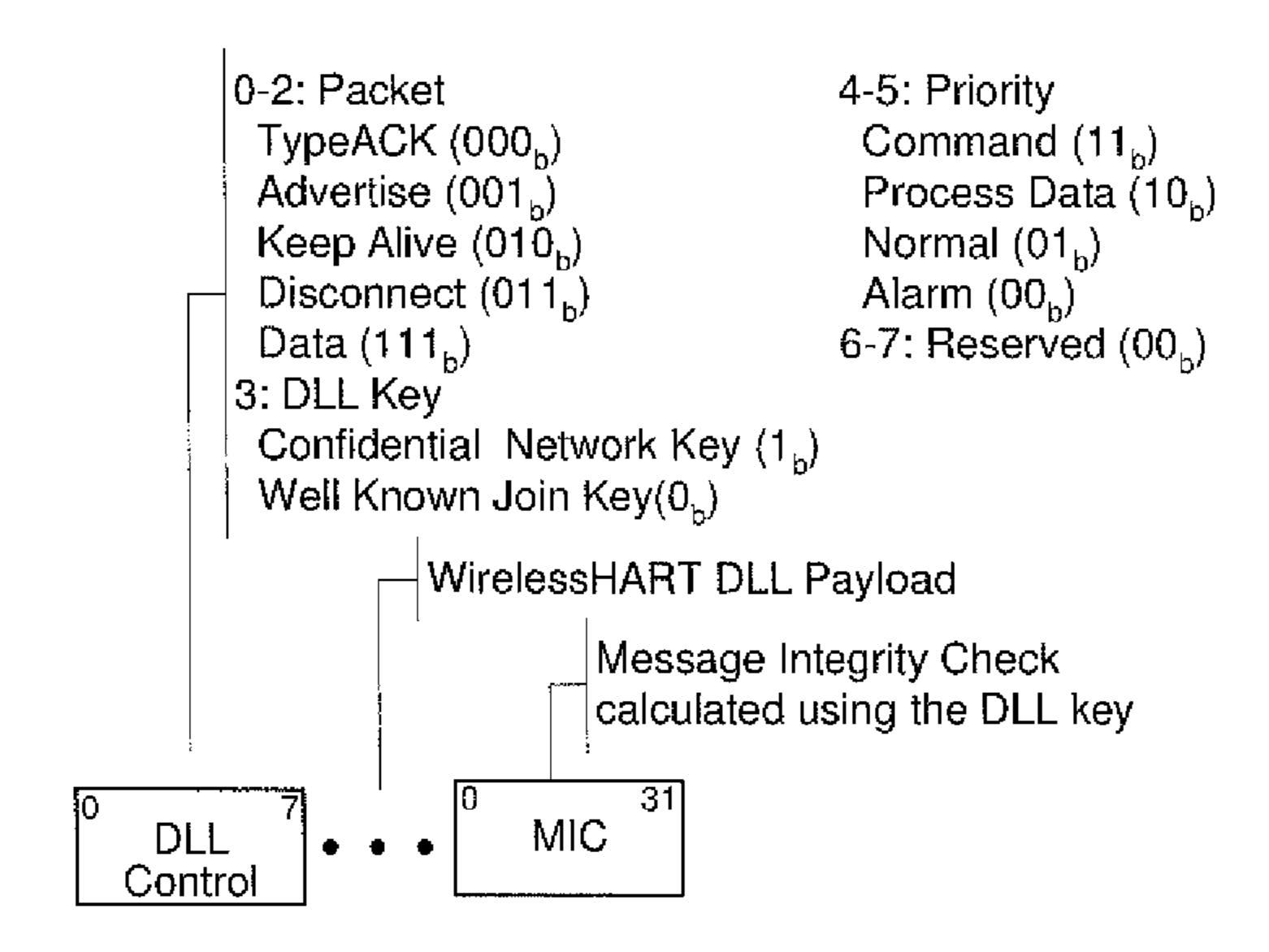
FIG. 5 Wireless HART DLL Header
