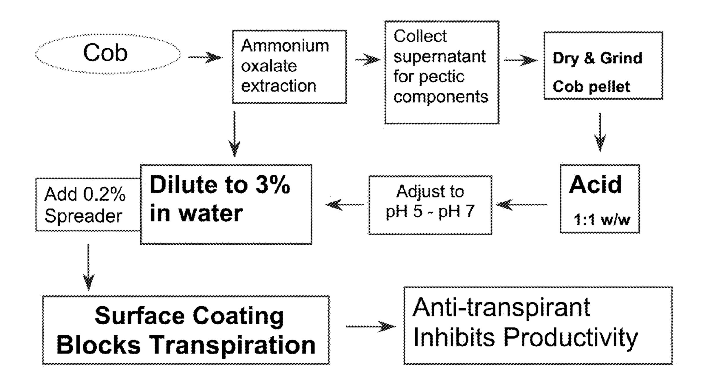
Figure 3. Process for integration of surface coating into PectiC<sup>+</sup>.
