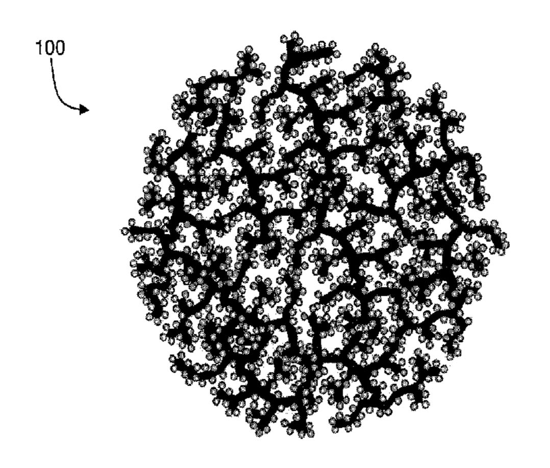
formed from a dendritic particle, which is a three-dimensional, randomly-ordered assembly of nanoparticles of an electrically conducting material and a plurality of discrete non-porous nanoparticles of a non-carbon Group 4A element or mixture thereof disposed on a surface of the dendritic particle. At least one nanocomposite of the plurality of
