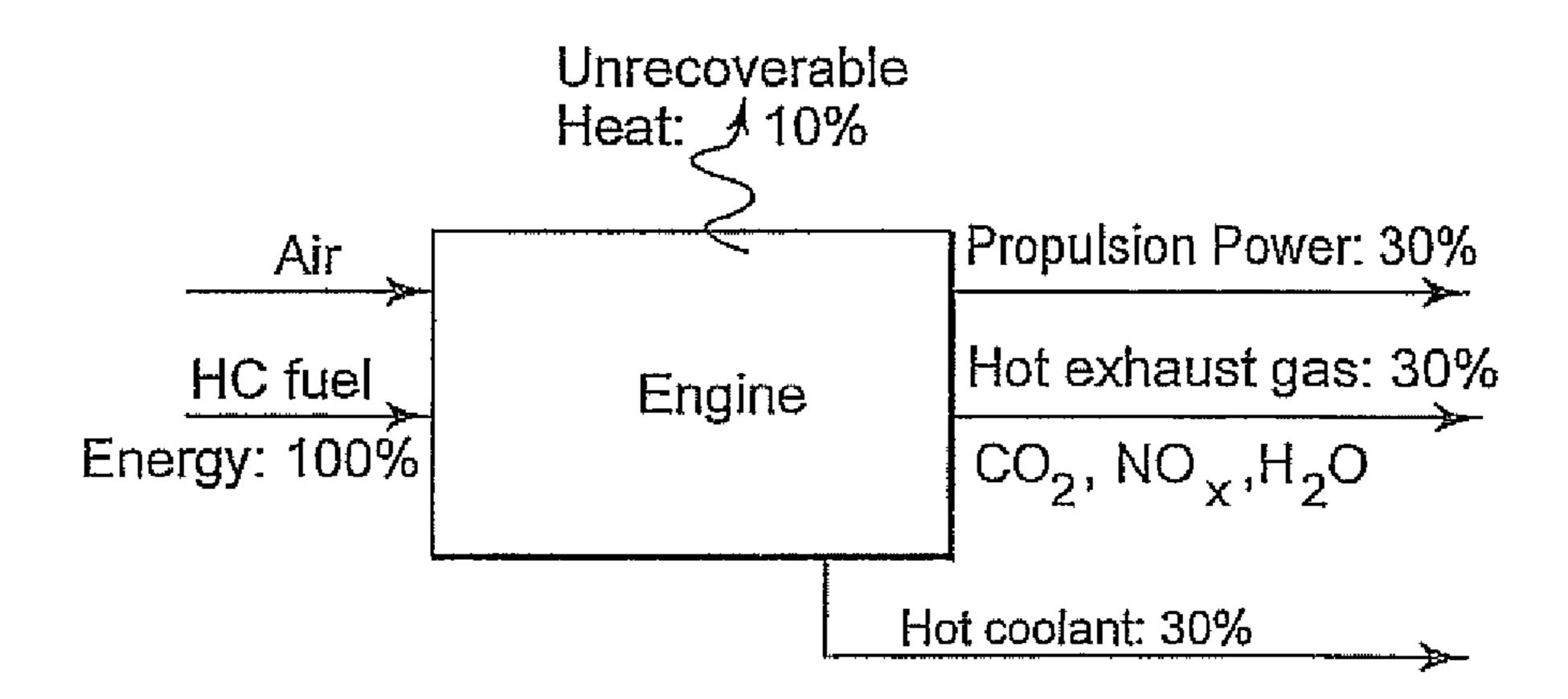
compression and/or pressurization, compression and/or refrigeration for densification of CO recovered from membrane module Conversion of heat to power for capture in membrane Propulsion Power: 30% Hot exhaust gas: 30%  $CO_2$ , NO  $_{\times}$ , H<sub>2</sub>O Hot coolant: 30% Unrecoverable Heat: ✓ 10% Engine HC fuel Energy:100%
