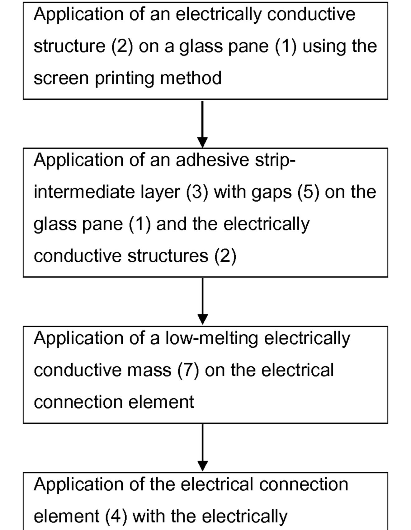
Mechanical and electrical connection of the parts at 110 ℃ by means of thermal activation.
