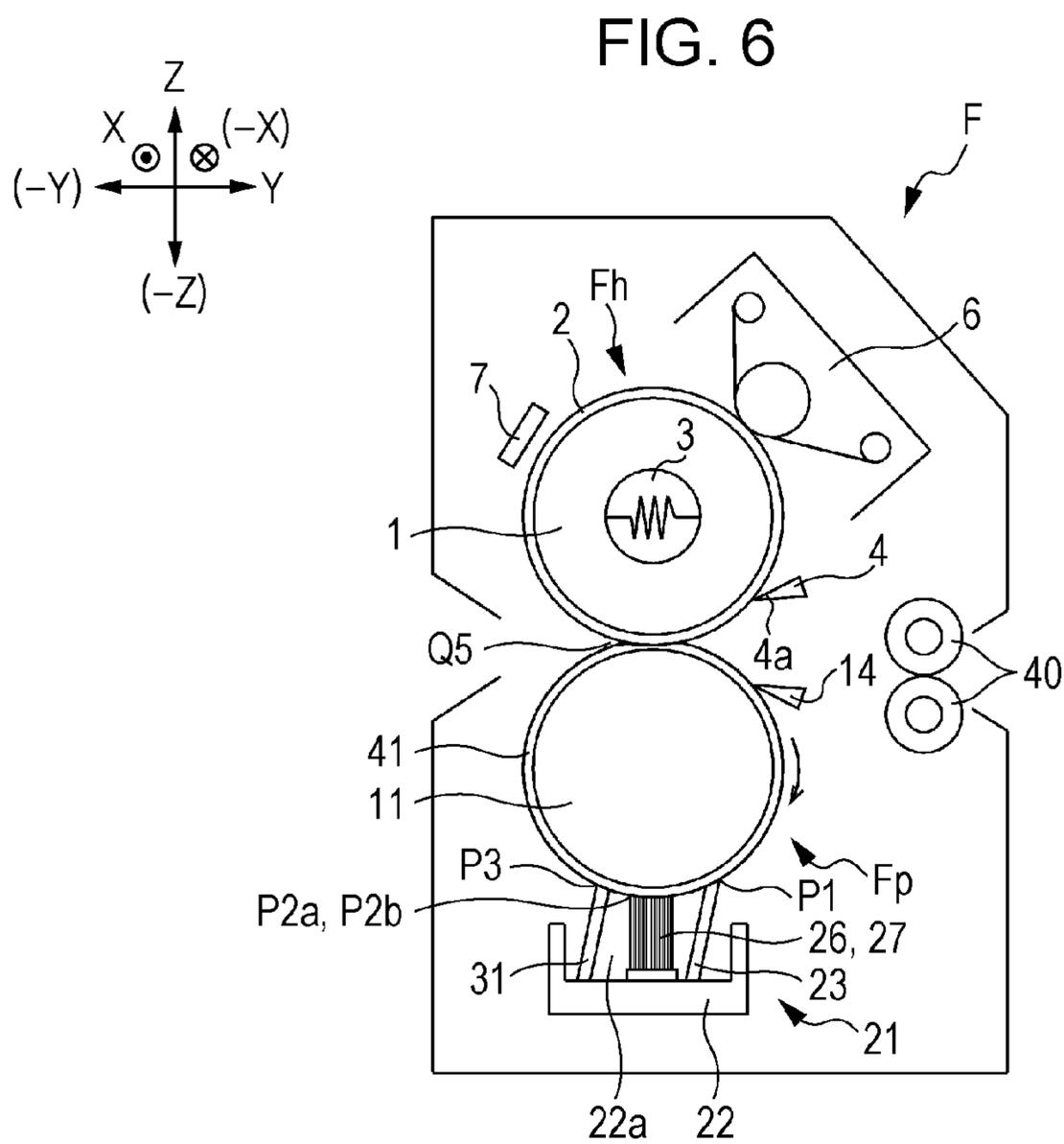
**1****FIXING DEVICE WITH ANTISTATIC AGENT
