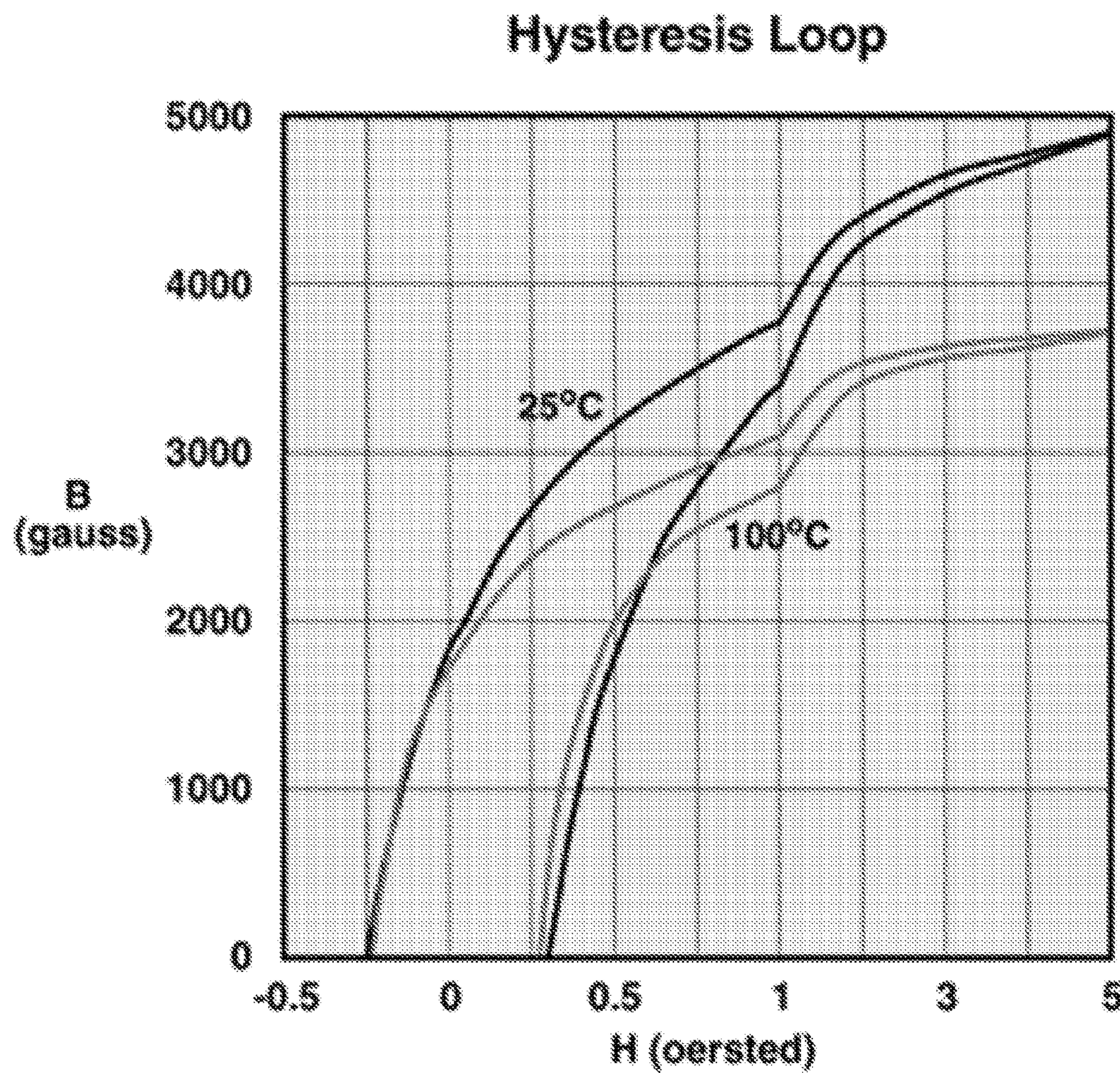
Measured on an 18/10/6mm toroid at 10kHz.
