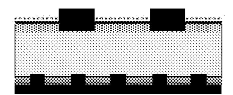
6. Screen printing of the front and back surfaces Co-firing
