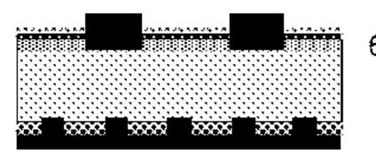
Screen printing of the front and back surfaces Co-firing
