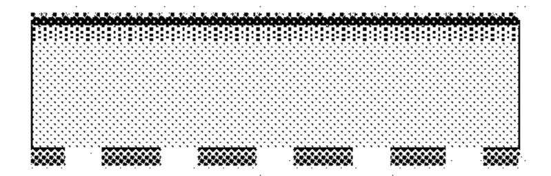
5. Opening of the passivation layer (SiO<sub>2</sub>/SiN<sub>x</sub> or Al<sub>2</sub>O<sub>3</sub>/SiN<sub>x</sub>) using SolarEtch<sup>®</sup> AQS
