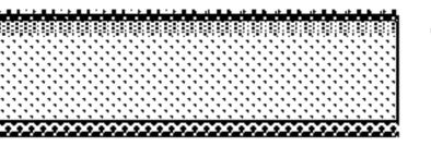
4. Deposition of the passivation layer (SiO<sub>2</sub> or Al<sub>2</sub>O<sub>3</sub>) and PECVD SiN<sub>x</sub>
