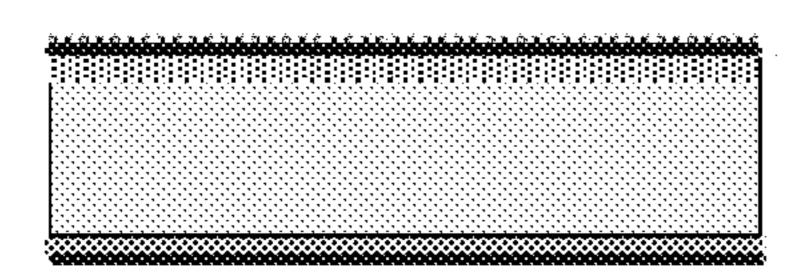
Deposition of the passivation layer (SiO<sub>2</sub> or Al<sub>2</sub>O<sub>3</sub>) and PECVD SiN<sub>x</sub>
