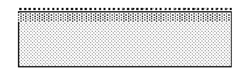
3. Back surface polishing and edge insulation (in one process step using etching paste) and PSG etching
