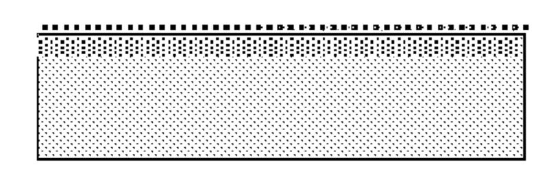
3. Back surface polishing and edge insulation (in one process step using etching paste) and PSG etching
