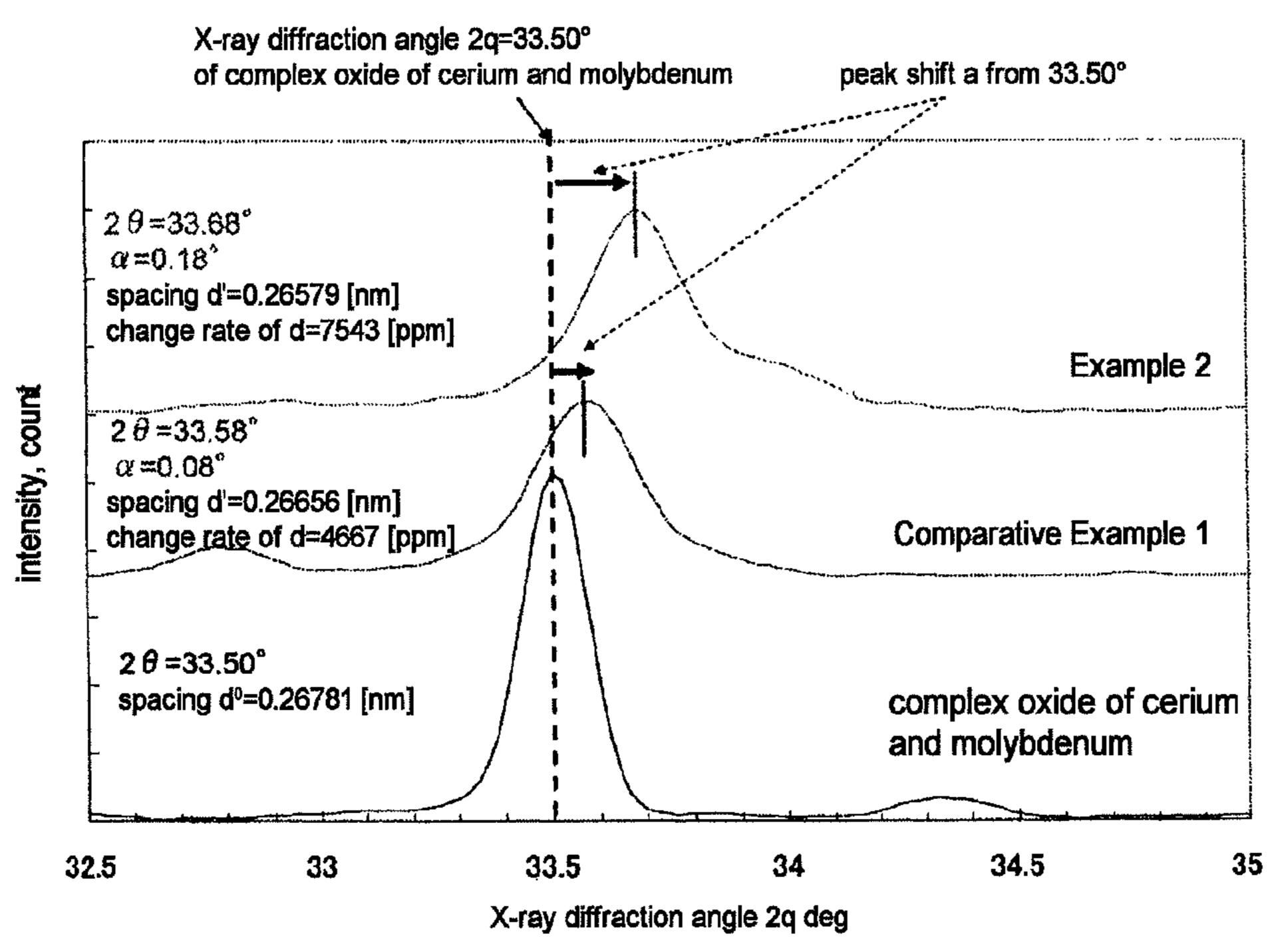
X-ray diffraction, enlarged view of X-ray diffraction angle 2q=32.5 to 35°
