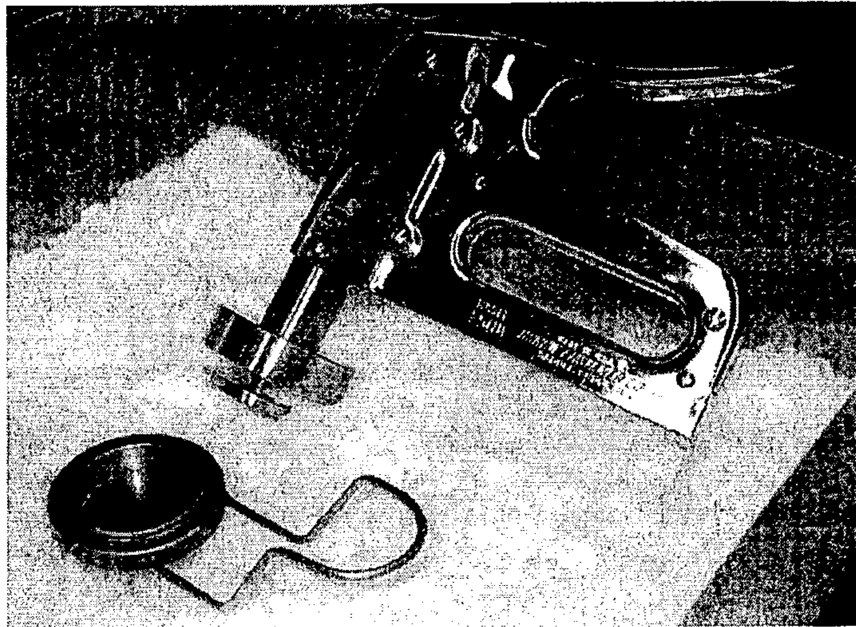
Figure 3 A custom-made staple gun for pulverizing frozen tissue.
