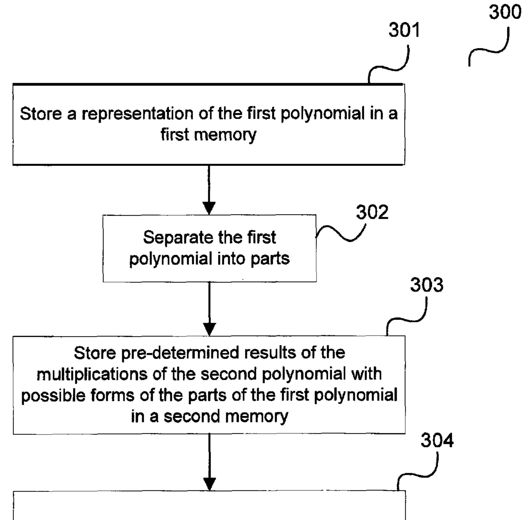
Determine, for each part of the first polynomial, a start address of a memory block of the second memory based on the form of the part and the location of the part within the first polynomial
