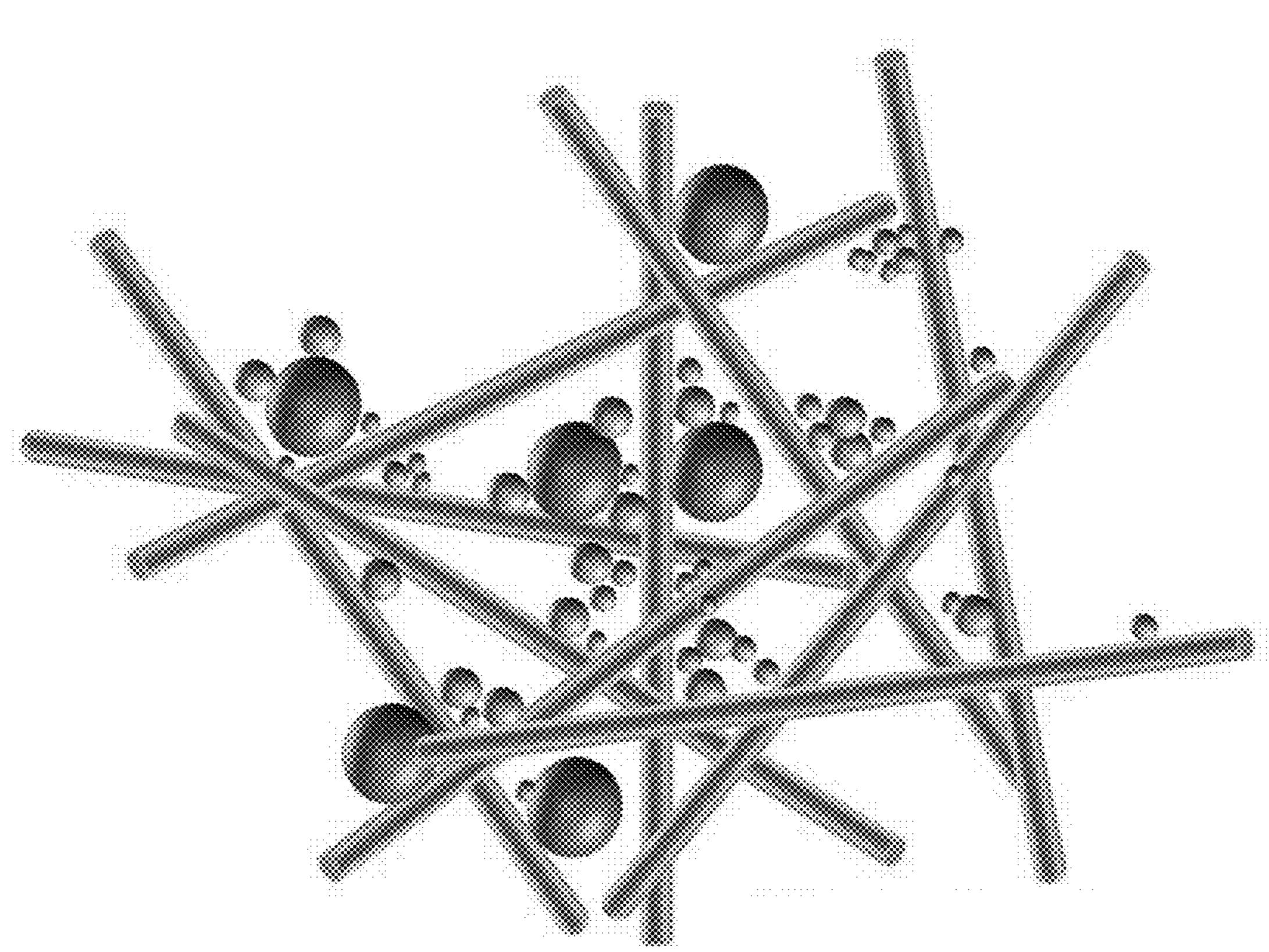
(500) Metal oxide nanofiber-nanoparticle-microparticle composite sensing material
