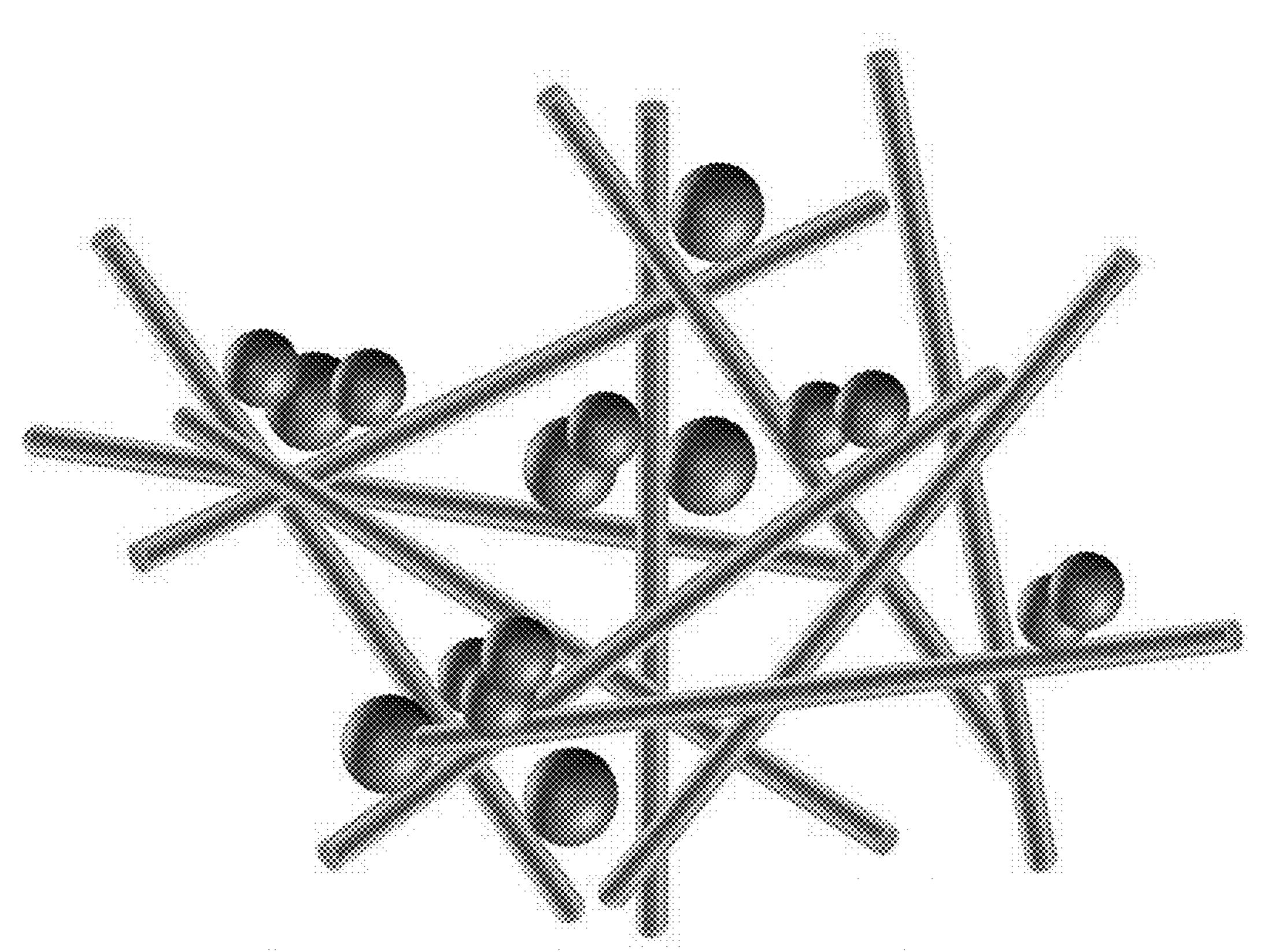
(600) Metal oxide nanofiber-microparticle composite sensing material
