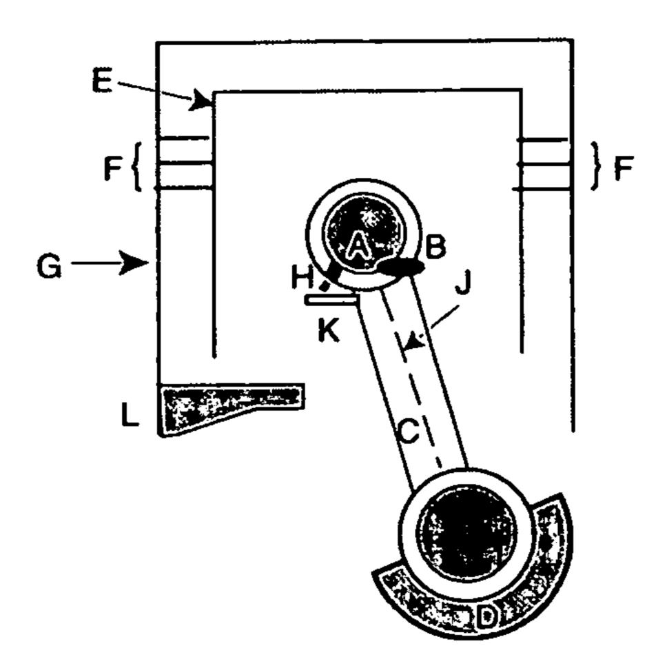
Detail of wrist pin and cleave deployment assembly
