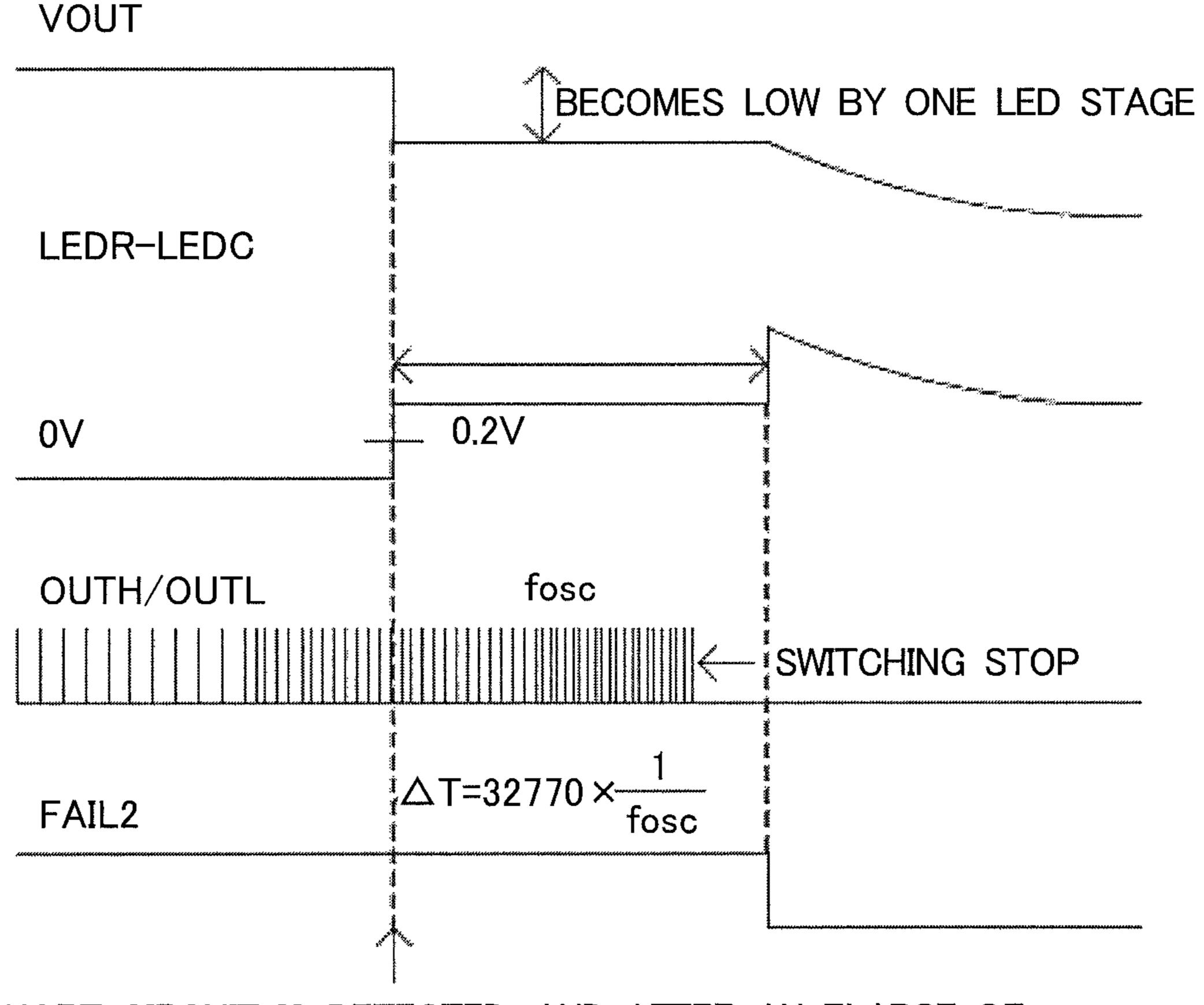
SHORT-CIRCUIT IS DETECTED, AND AFTER AN ELAPSE OF A TIMER TIME OF  $\Delta T$ , TROUBLE IS DETECTED BY MEANS OF FAIL2
