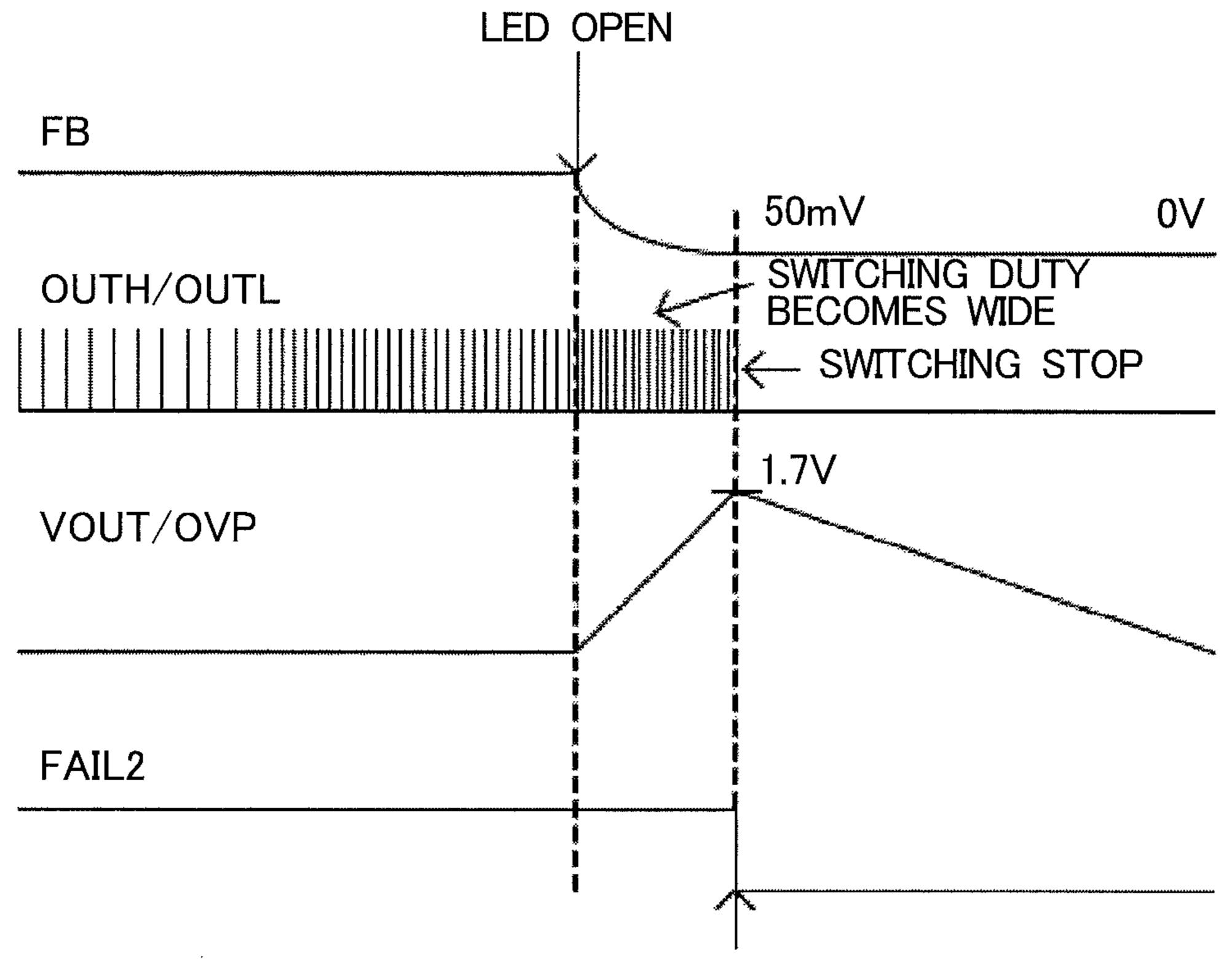
LED OPEN DETECTION UNDER VOVP $\ge$  1.7 AND VFB  $\le$  50 MV (FP LATCH IS PERFORMED WHEN DETECTION CONDITION IS MET)
