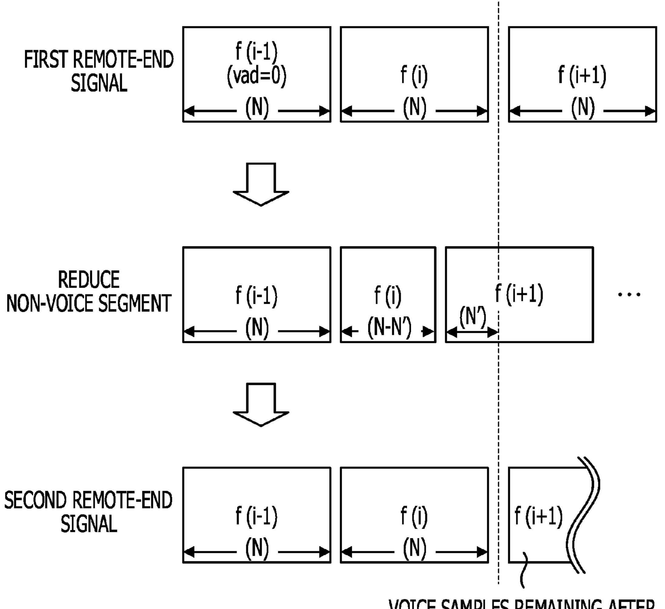
VOICE SAMPLES REMAINING AFTER REDUCTION OF NON-VOICE SEGMENT ARE TRANSMITTED IN f(i+1) TOGETHER WITH PART OF VOICE SAMPLES OF f(i+2)
